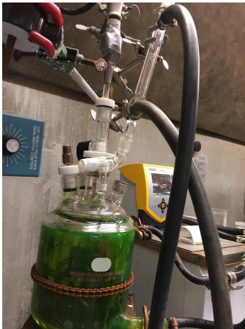
Figure 3.2 Jacketed vessel reactor apparatus setup for condensation reactions conducted in LORRE.
