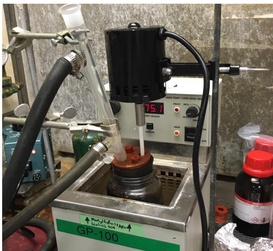
Figure 3.1 Standard water bath apparatus setup for condensation experiments conducted in LORRE.
