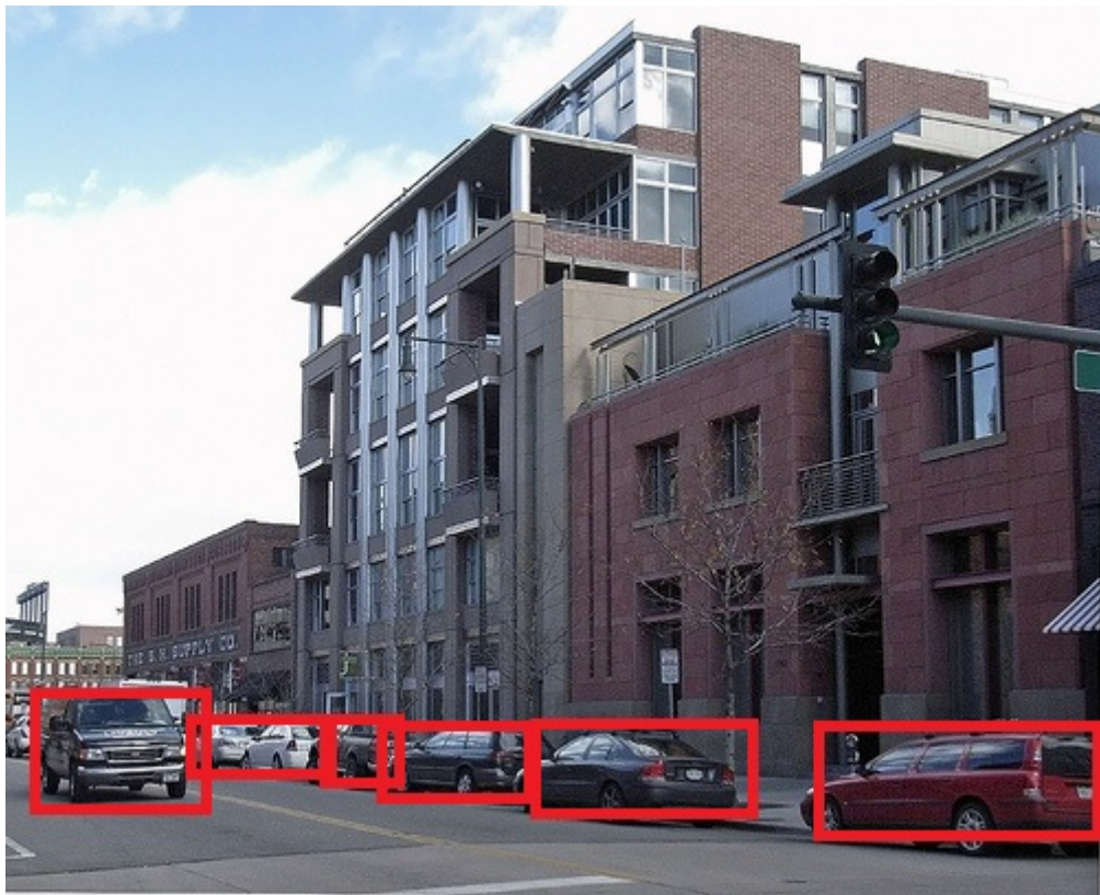
Figure 2.6. An example of Fast R-CNN detecting cars in an image from (R. Girshick, 2015).
