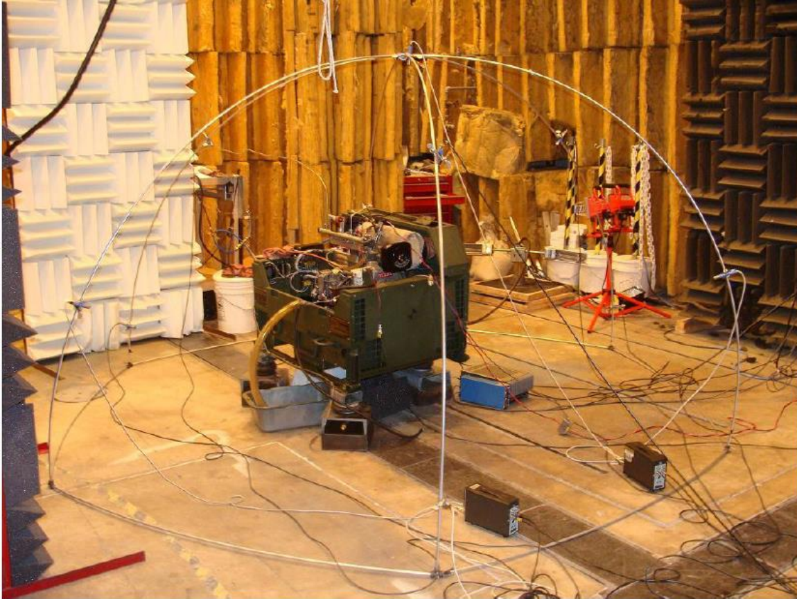
Figure 3.4. Sound pressure measurement setup in hemi-anechoic chamber [2].
