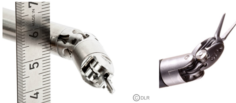
Figure 2.6. Cable driven end-effectors: Link driven multiple DOF forceps (Left) [7] and Endowrist needle driver (Right) [17].
