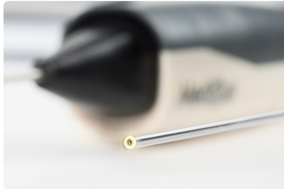
Figure 3.7. Medigus microScout camera (2 mm diameter) [21].
