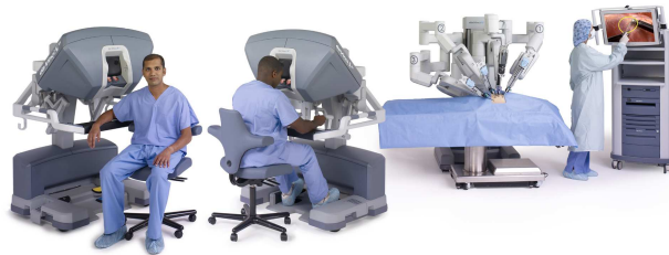
Figure 2.1. Intuitive surgical da Vinci Surgical System [18].
