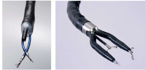
Figure 2.2. Devices for NOTES surgery: Boston Scietific DDES (Left) and Olympus Corp. EndoSAMURAI (Right) [33].
