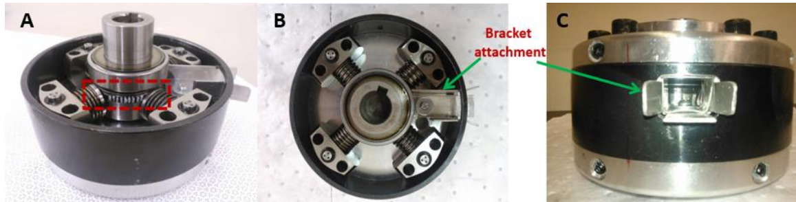
Figure 35: (A) Painted outer race, (B) Custom bracket attachment used in the test rig setup, (C) Camera view during measurements.
