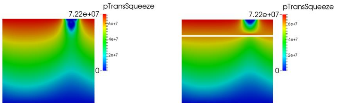
Figure 57: Comparison between the pressures generated from the translational squeeze effect for the case of a piston with no grooves (left) and a piston with grooves at Position A (right) during one instant of the discharge stroke.
