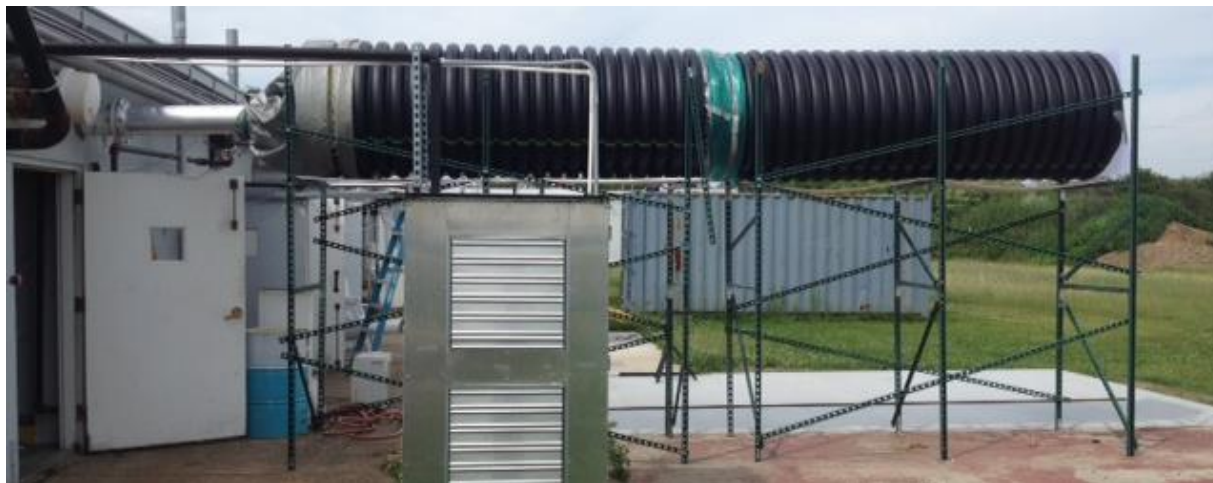
Figure 4.11: Second Configuration of Settling Chamber with 20 Foot Length.
