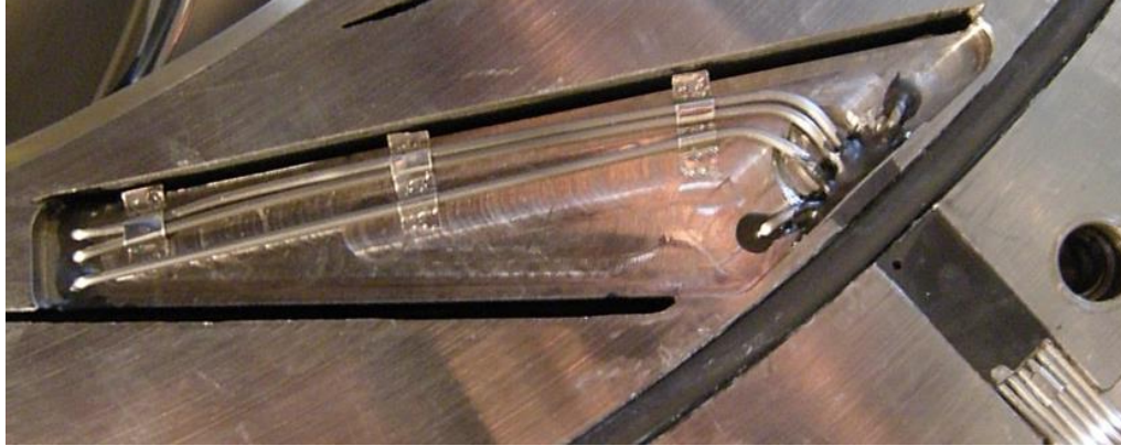
Figure 2.16: External View of the Diffuser Vane Passage Static Taps.
