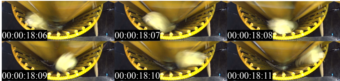
Figure 31 - Six frames from video footage of a cob moving around the threshing cylinder.
