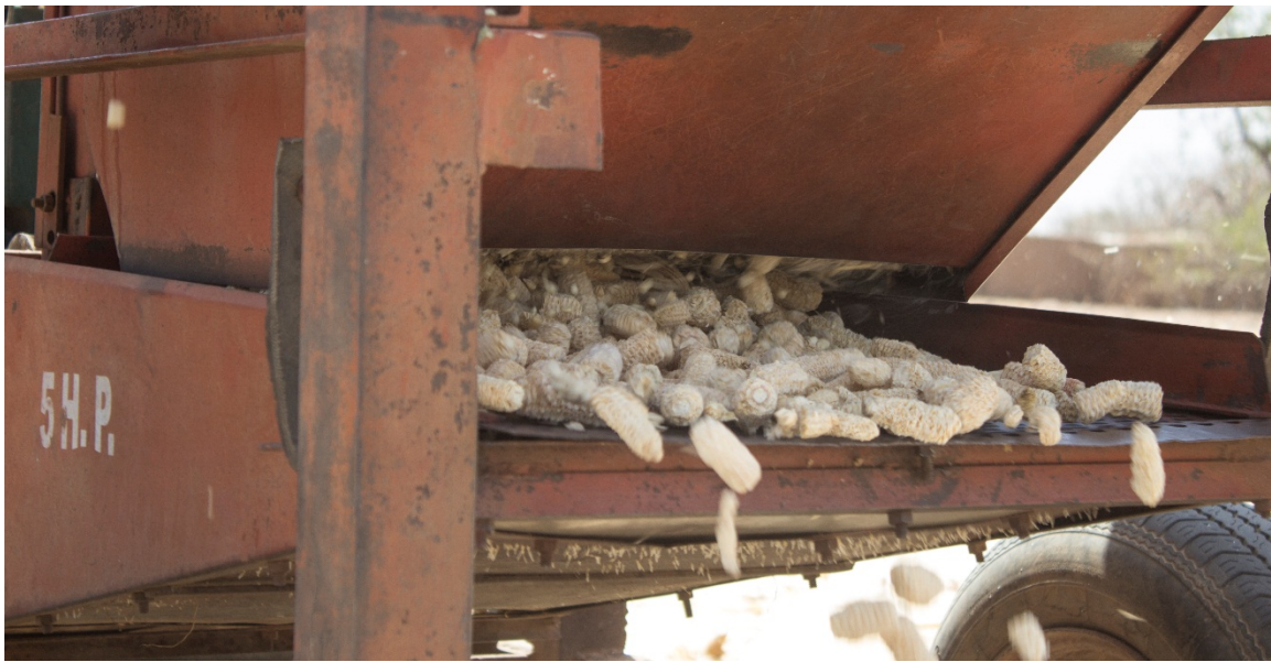
Figure 4 - A thresher in Ghana threshing corn. The cleaning sieve becomes overloaded with corncobs, causing grain loss. Source: Author.
