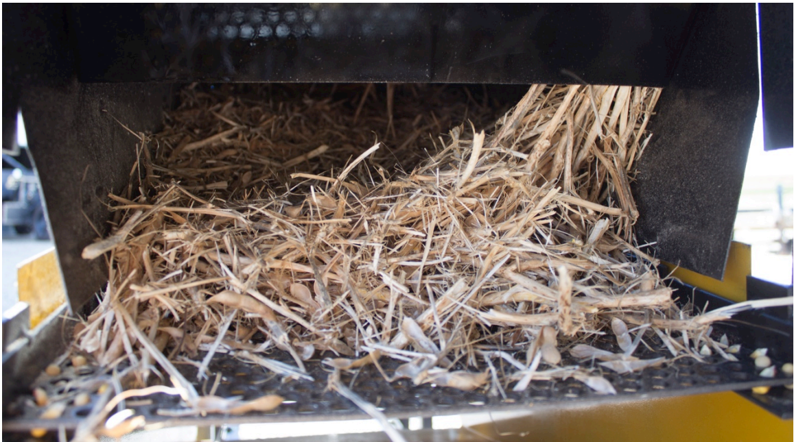
Figure 23 - Picture of the overloaded sieve after the initial soybean test. Source: Author.
