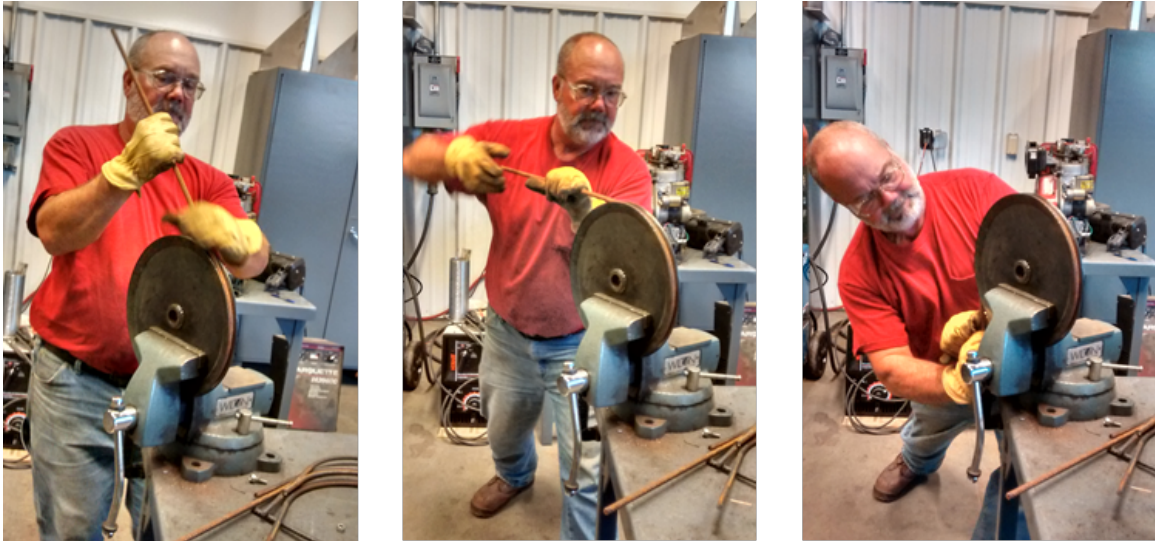
Figure 16 - A series of photos showing how the rebar was bent into an arc. Source: Author.
