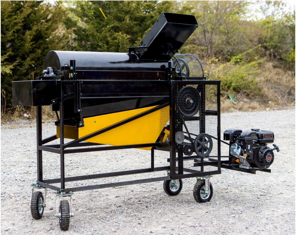
Figure 20 - The final thresher before testing. Wheels were added to assist movement. Source: John Lumkes.
