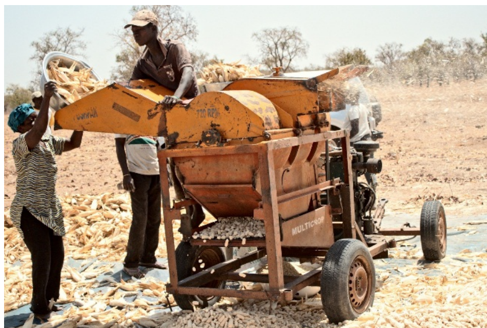
Figure 2 - A thresher in Ghana shelling corn. Source: Author.
