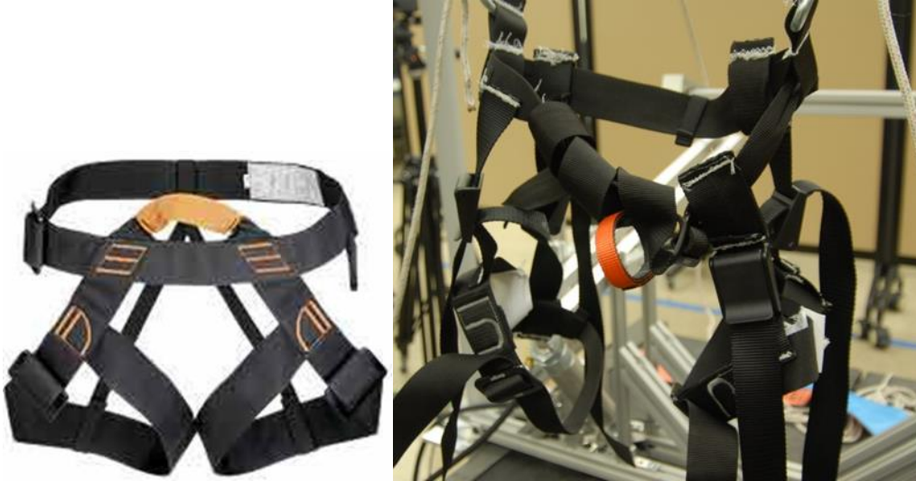
Figure 22. The standard rock climbing harness, on the left, and the modified harness attached to the apparatus, on the right.
