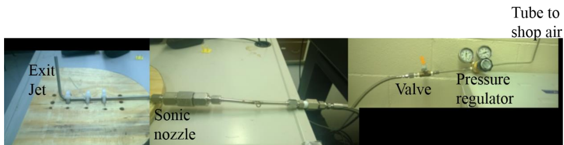
Figure 5-1: Experimental apparatus for sonic nozzle flow test.
