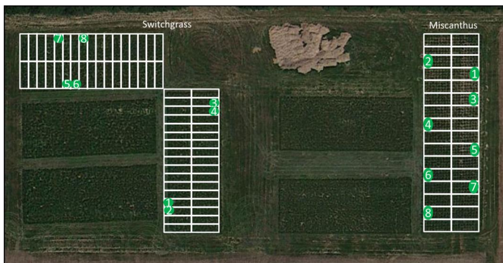
Figure 3.2 TPAC West perennial grass experiments; locations of lysimeters are shown and numbered sequentially by replicate (e.g. replicate 1, lysimeter 1 & 2).
