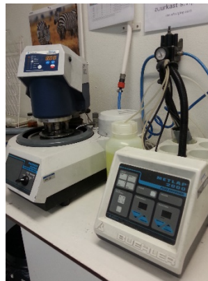
Fig 7-2 Automatic polisher (Bubler vector power head and phoenix alpha grinder)
