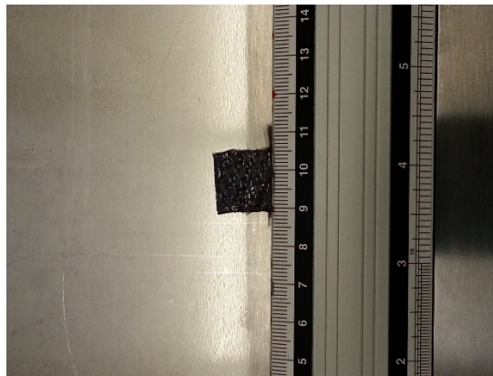
Fig 4-3 Discontinuous carbon-PPS flake
