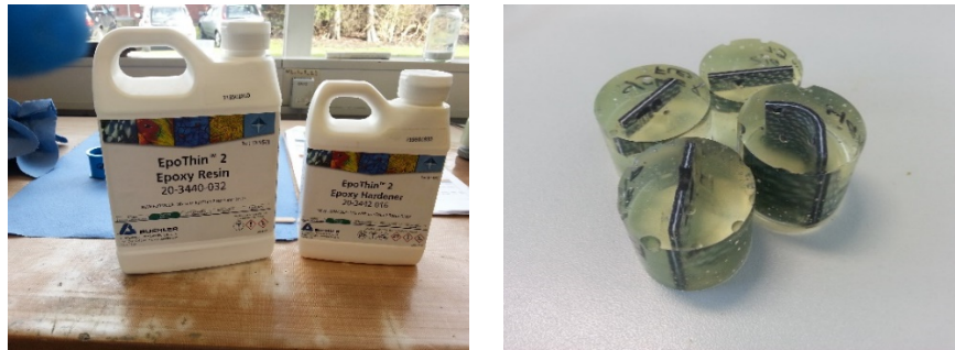
Fig 7-1 Epoxy-Hardener system and samples cured in the mixture
