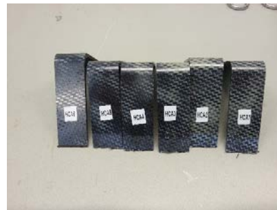
Fig 4-11 Samples made after cutting using diamond saw
