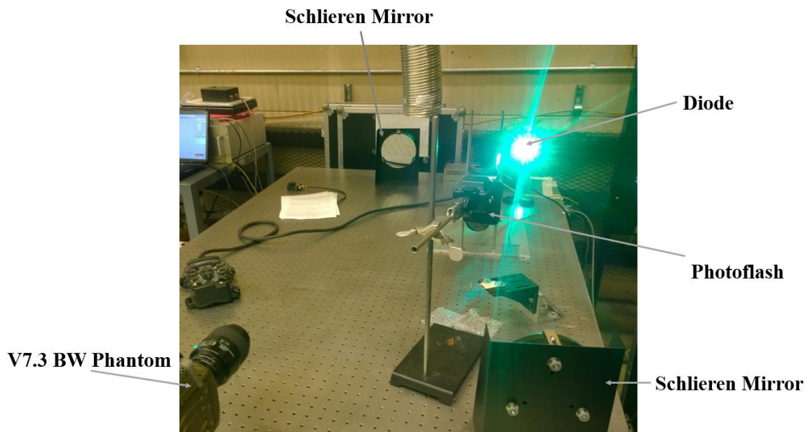
Figure B. 2 Set-up of the flash ignition experiment (front view)
