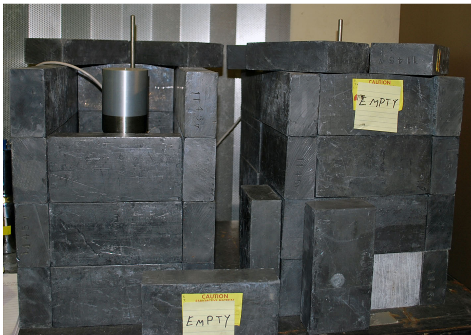
Figure 5.1. Each NaI well detector is housed in a 2-inch-thick lead cave. The sample vials are placed in the well for counting.
