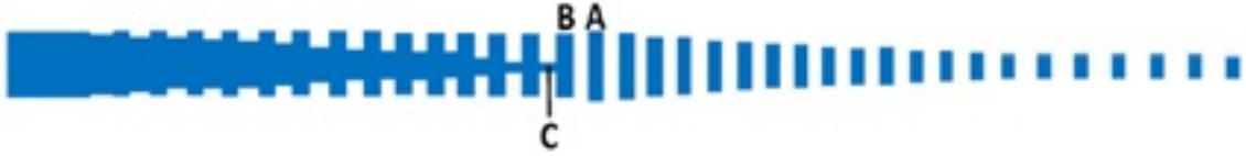
Fig. 2.20.: The structure of a Subwavelength Grating Waveguide (SWG) Taper [38]
