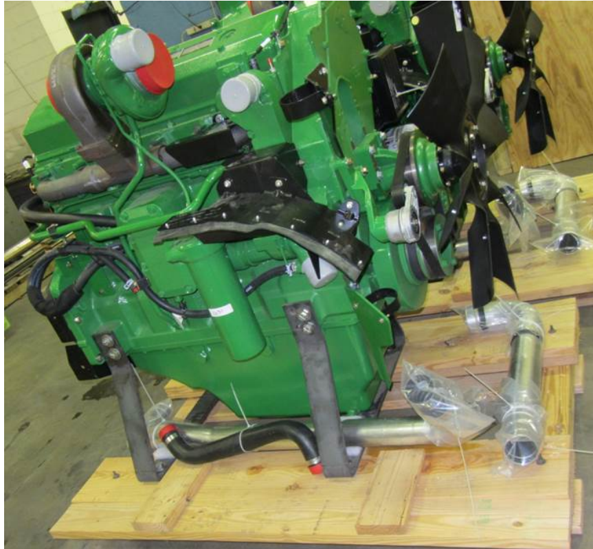
Figure 7.6. Example of placing minor SKD modules around the core SKD module(s) on the same pallet, forming pallet module (P-Module)
