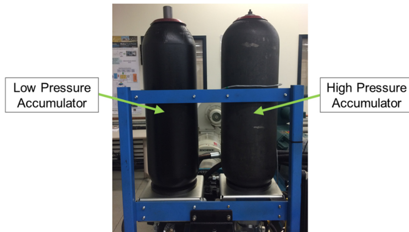
Figure 7.6: High and low pressure accumulators
