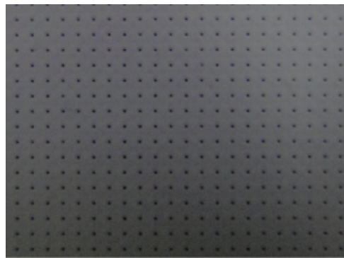
Figure 4.5. The microperforated panel (MPP) with a flow resistance of 454 Rayls.
