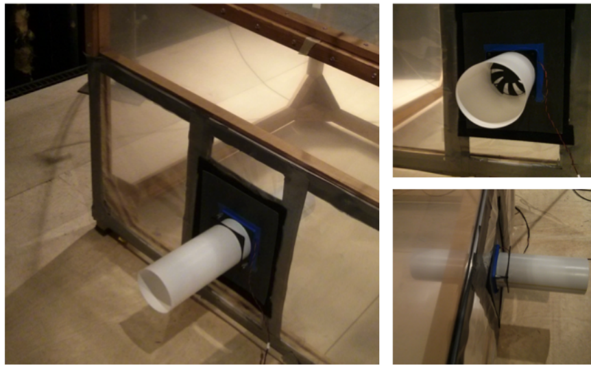
Figure 2.16. The actual photo of microperforated duct application to the axial fan noise testing.
