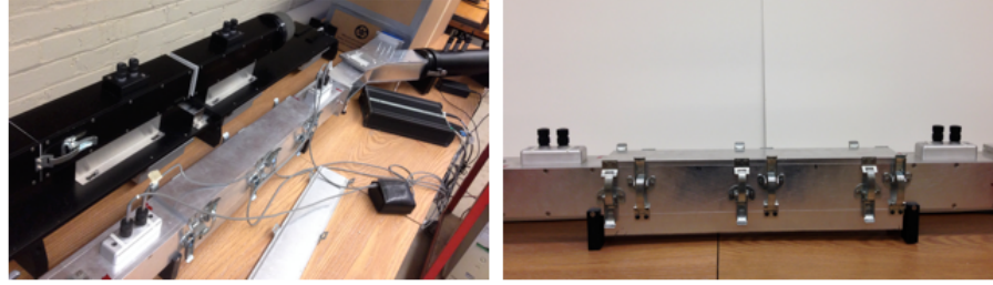
Figure 5.1. The square standing wave tube that was used for the measurements.
