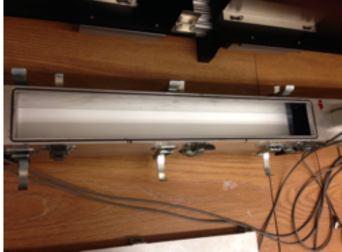
Figure 5.3. A picture of the MPP lining installation inside the square type standing wave tube.
