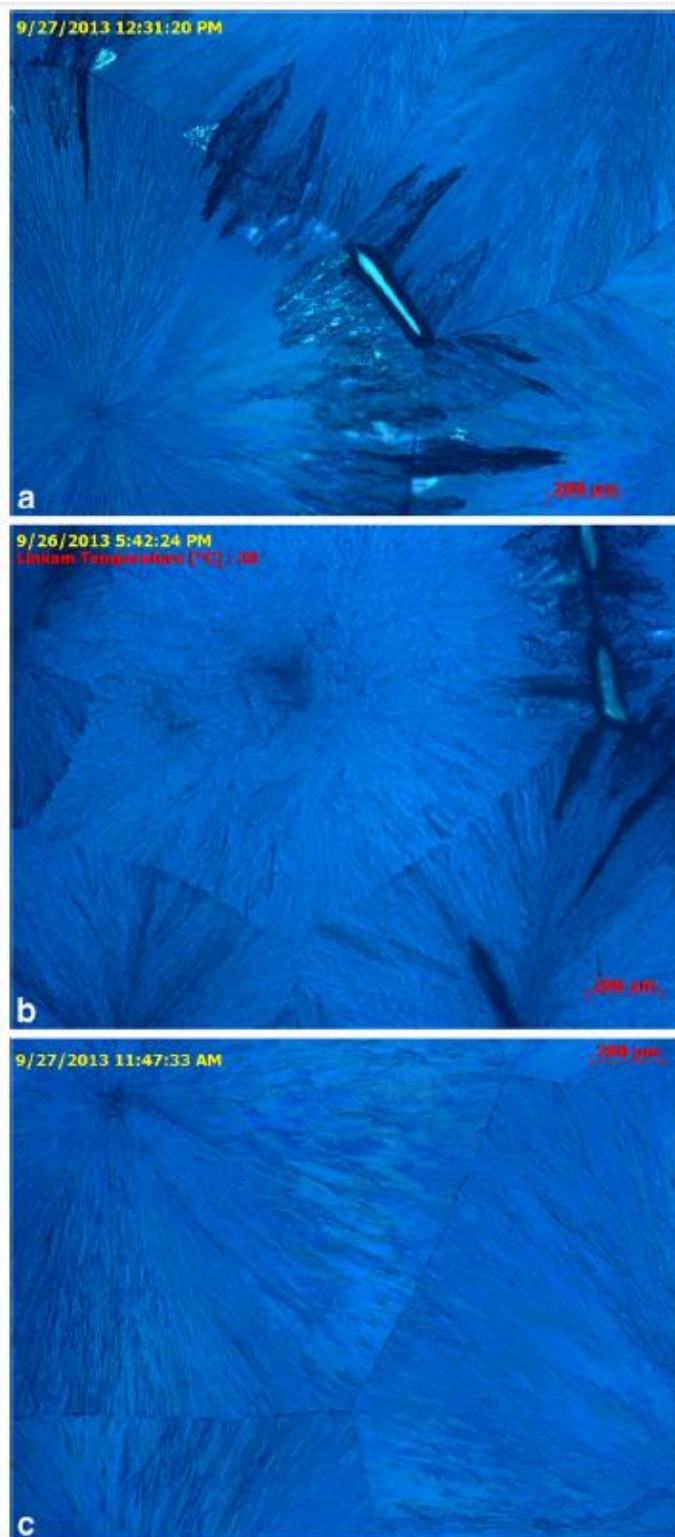
Figure 5.5 Optical microscopy images of melt-based deposits (Naproxen-PEG 3350) after a. fast cooling, b. slow cooling, c. cycling.
