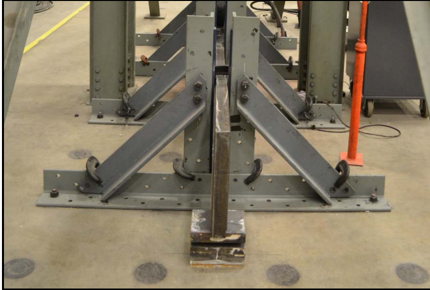
Figure 3.22: Axial fatigue test setup lateral bracing
