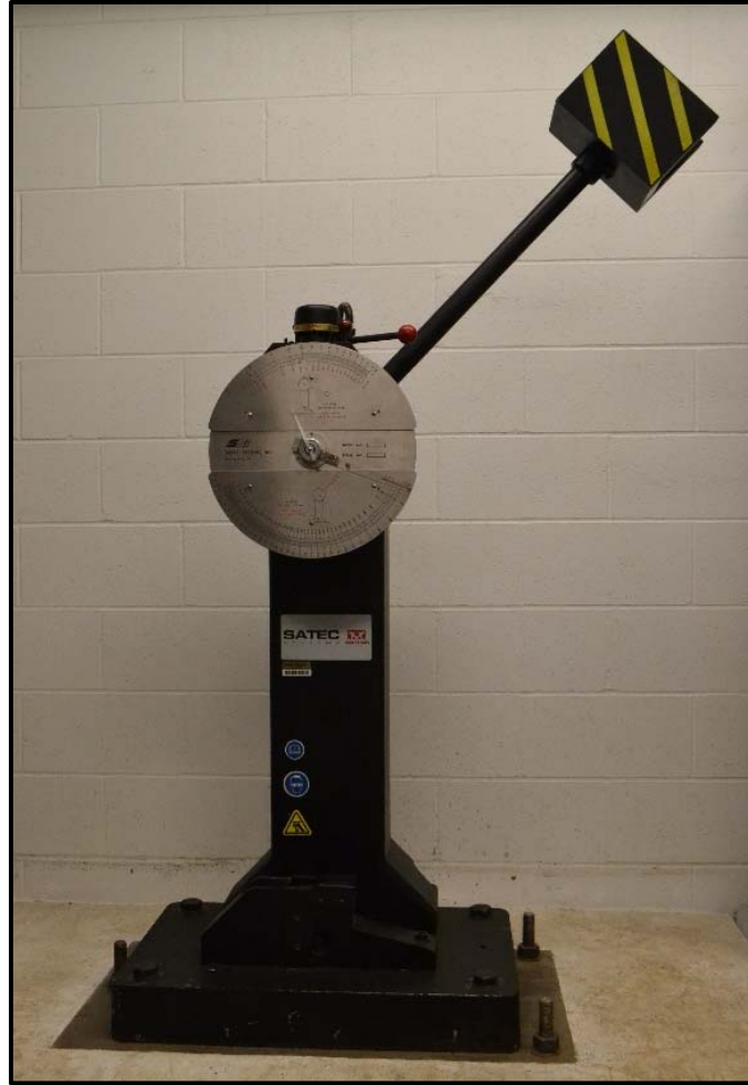
Figure 3.4: SATEC Series Impact Testing Machine
