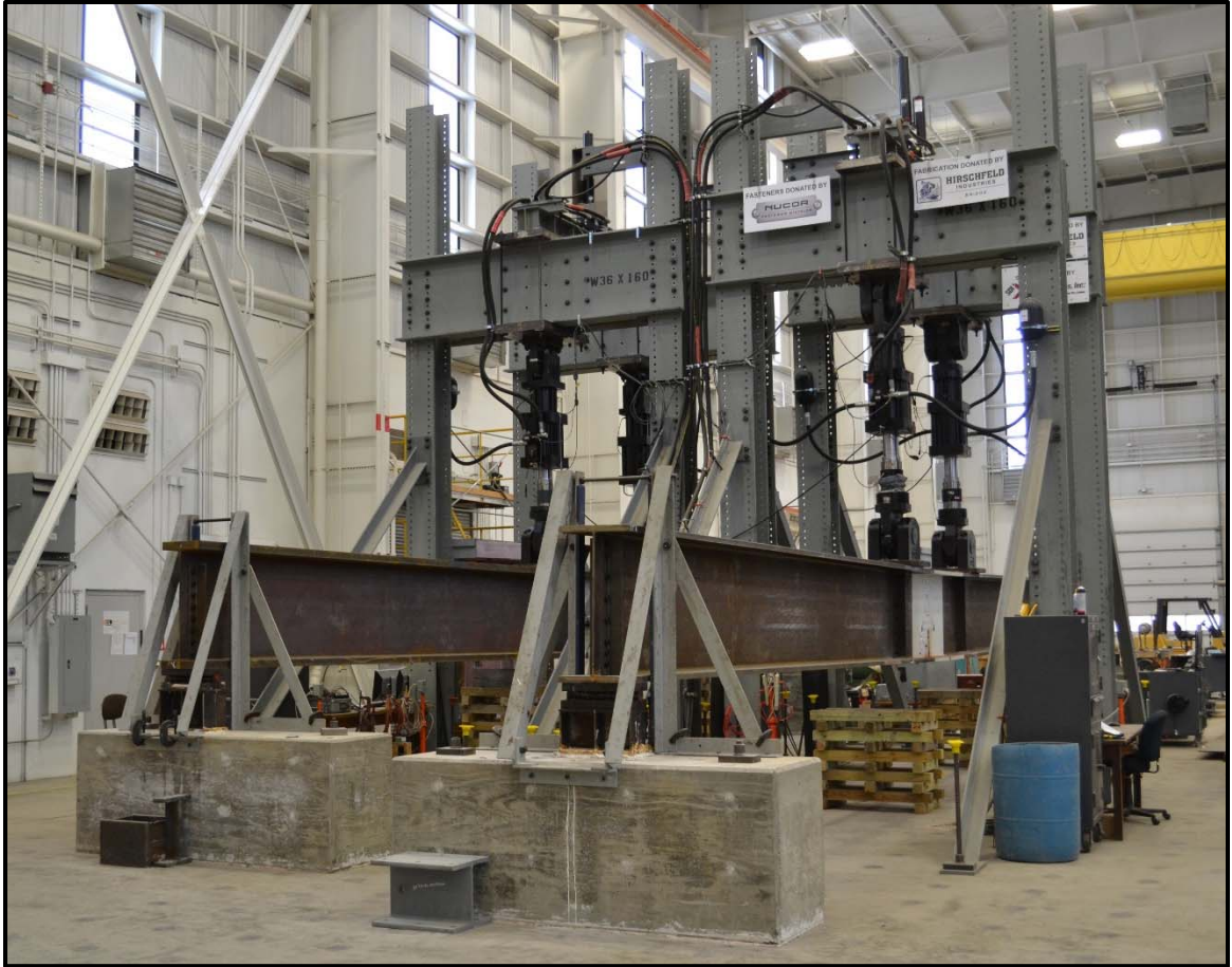
Figure 3.16: Twin bending test setups
