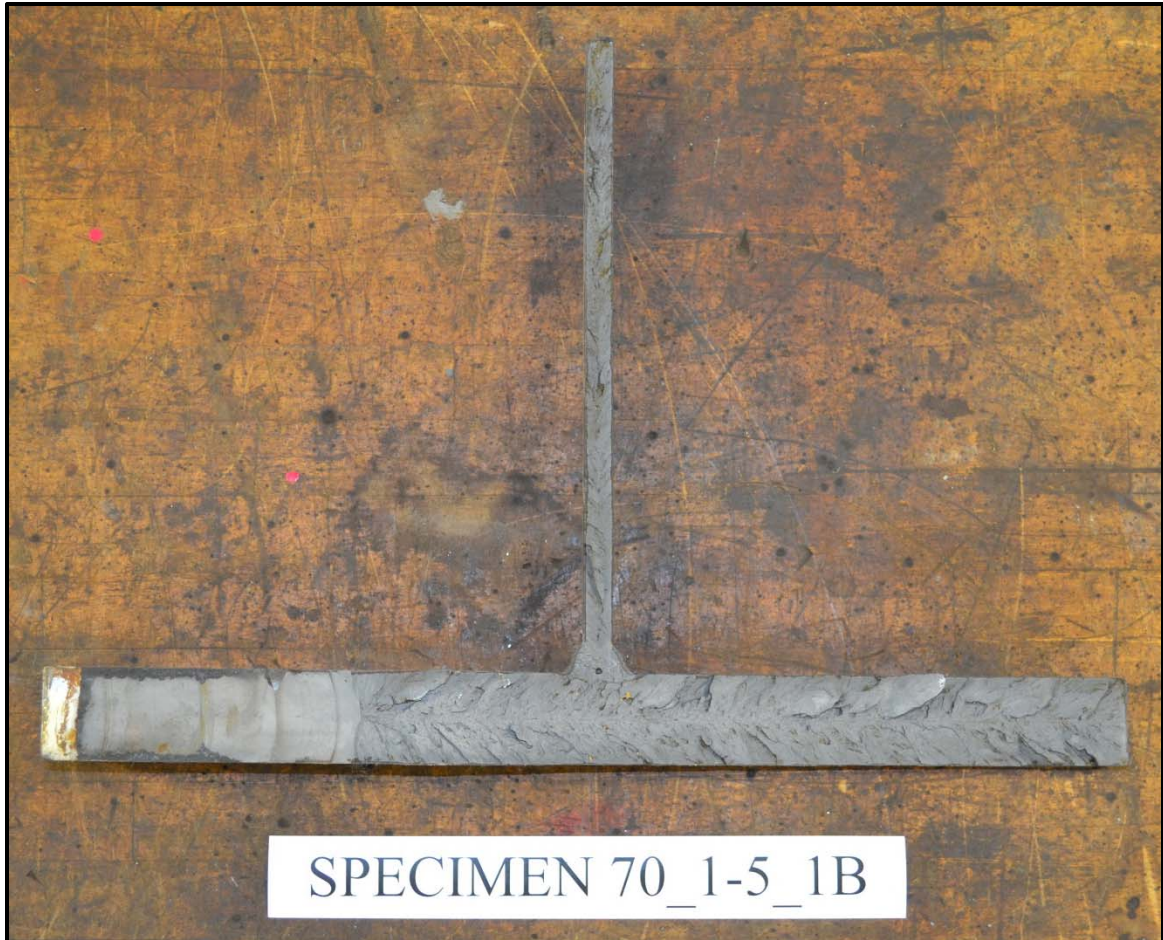
Figure 3.48: Specimen 70_1-5_1B fracture surface
