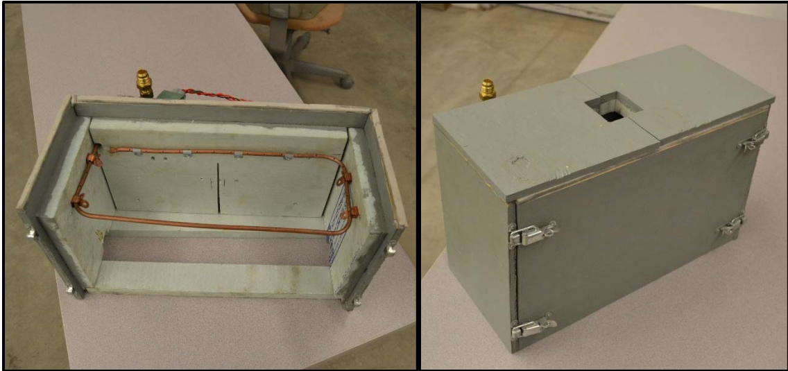
Figure 3.9: Fracture mechanics testing temperature chamber
