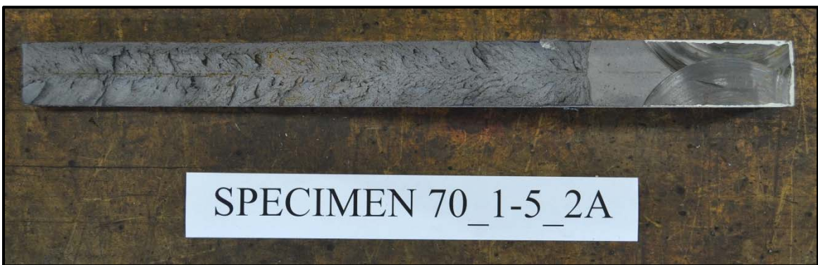
Figure 3.60: Specimen 70_1-5_2A fracture surface
