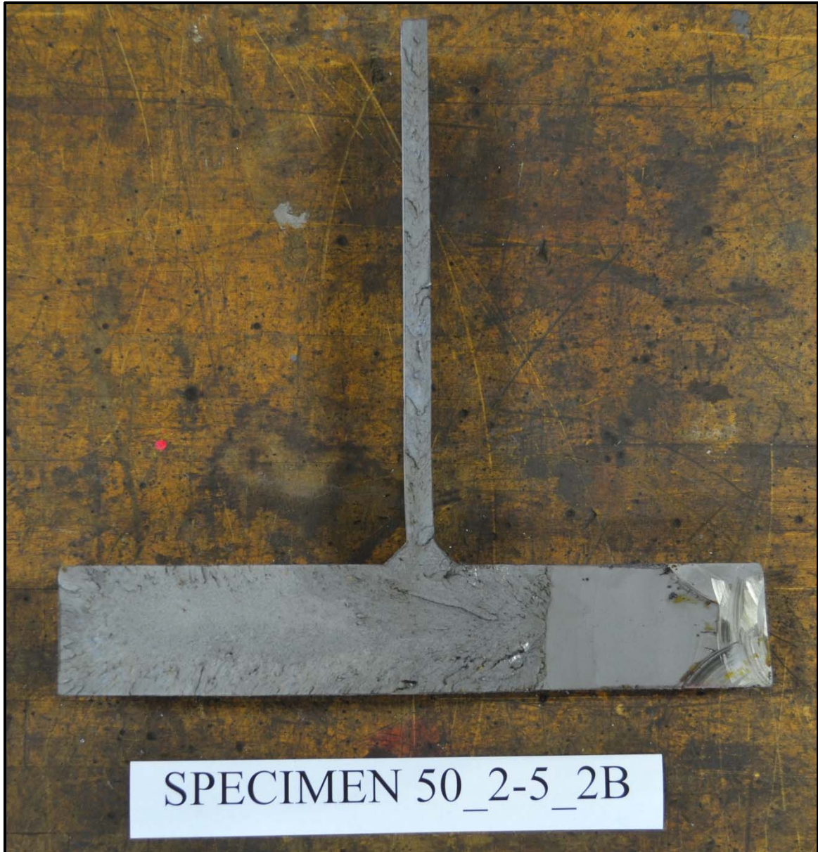
Figure 3.46: Specimen 50_2-5_2B fracture surface
