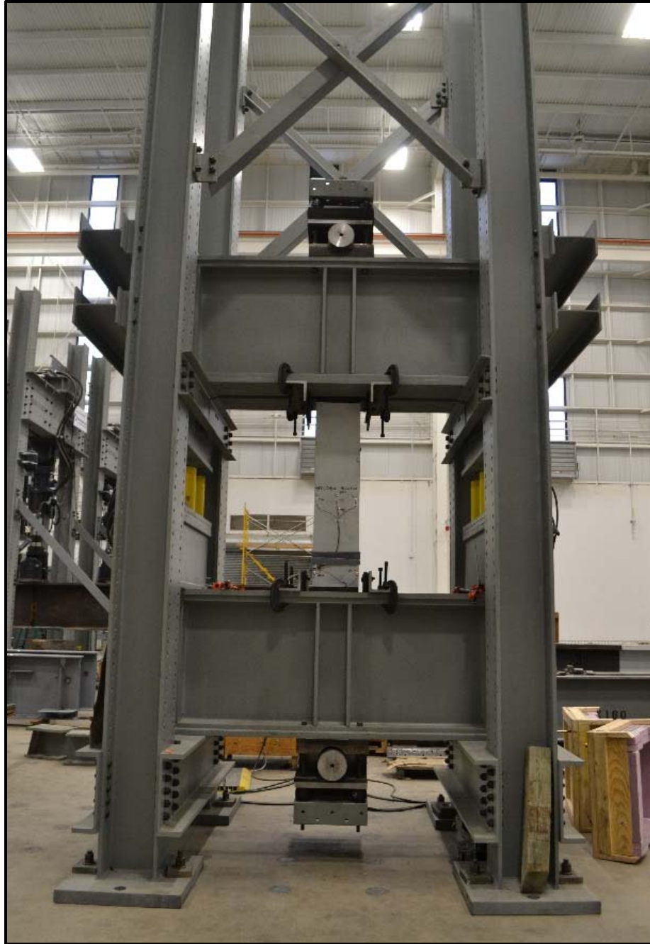
Figure 3.24: Axial test fracture setup
