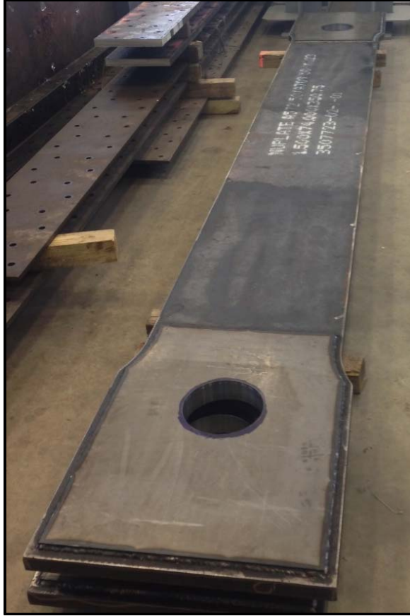
Figure 3.14: Representative axial test specimen
