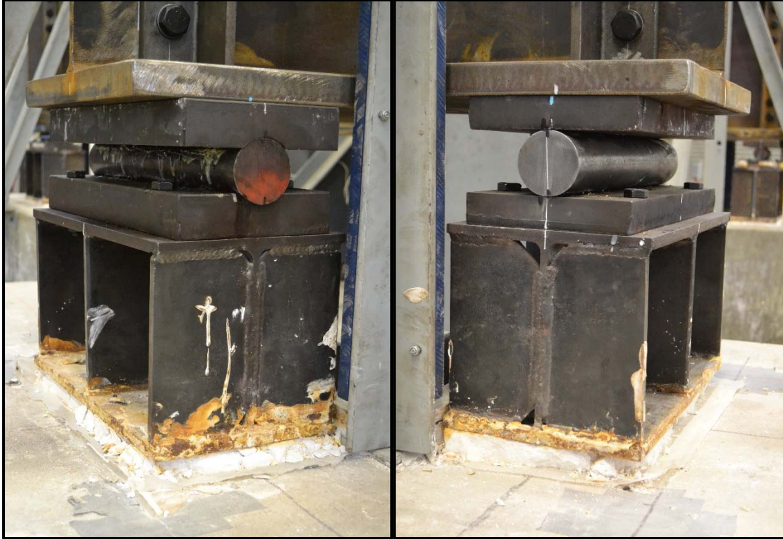
Figure 3.17: Pin bearing (left); Roller bearing (right)
