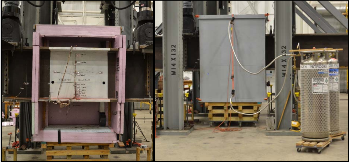
Figure 3.33: Bending temperature chamber
