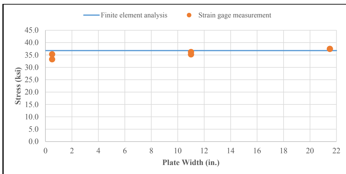
Figure 4.19: Specimen 50_1-5_1A longitudinal stress at midpoint
