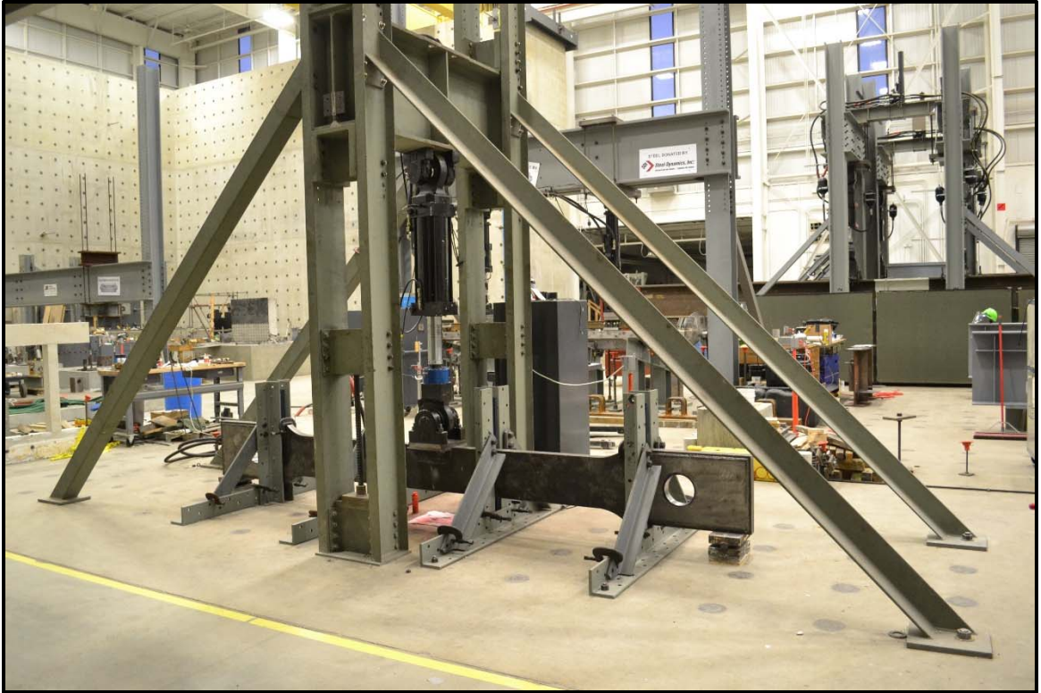
Figure 3.21: Axial test fatigue setup
