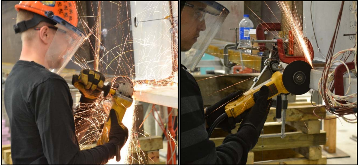
Figure 3.26: Straight notching (left); V-notching (right)
