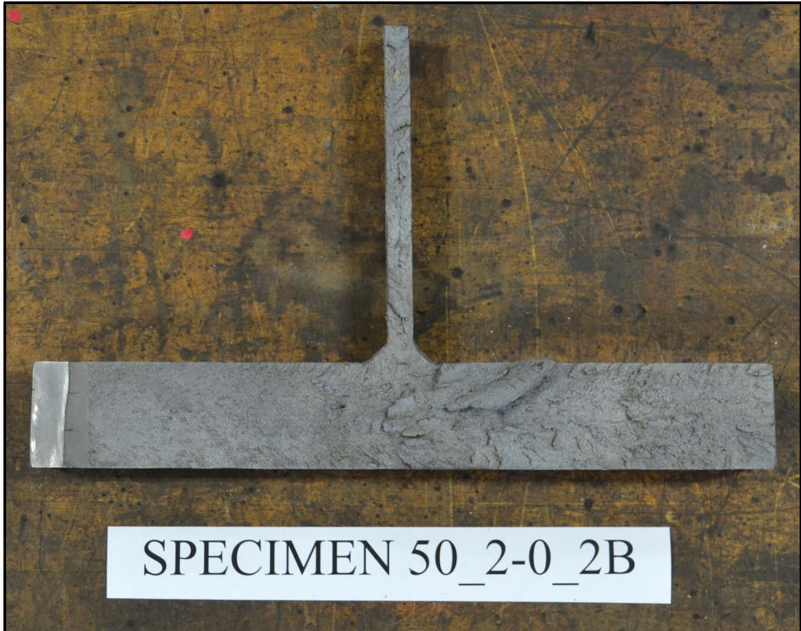
Figure 3.41: Specimen 50_2-0_2B fracture surface
