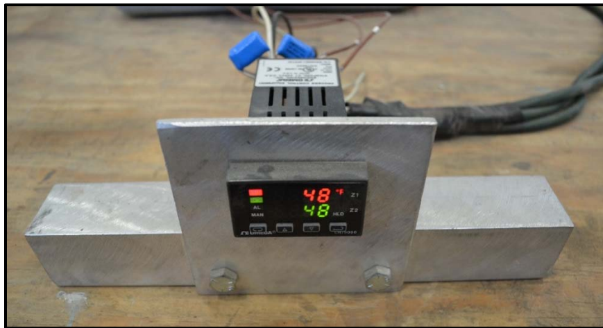
Figure 3.32: Dual zone temperature controller
