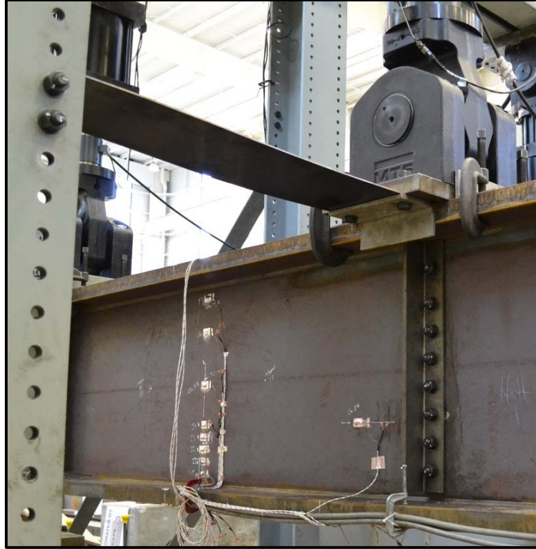
Figure 3.19: Lateral torsional buckling bracing
