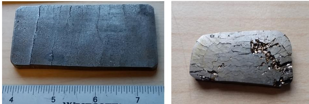
Figure 5-2 – Failed samples after 1 pass of cold rolling: (a) Fe-4wt%Si, (b) Fe-6.5wt%Si. Severe cracking is evident with cracks traversing the entire width of the specimens.
