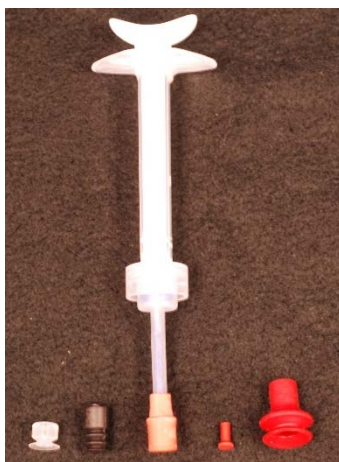
Figure 4.2. Dual barrel syringe with a variety of suction cups and the complete assembly with a suction cup attached.
