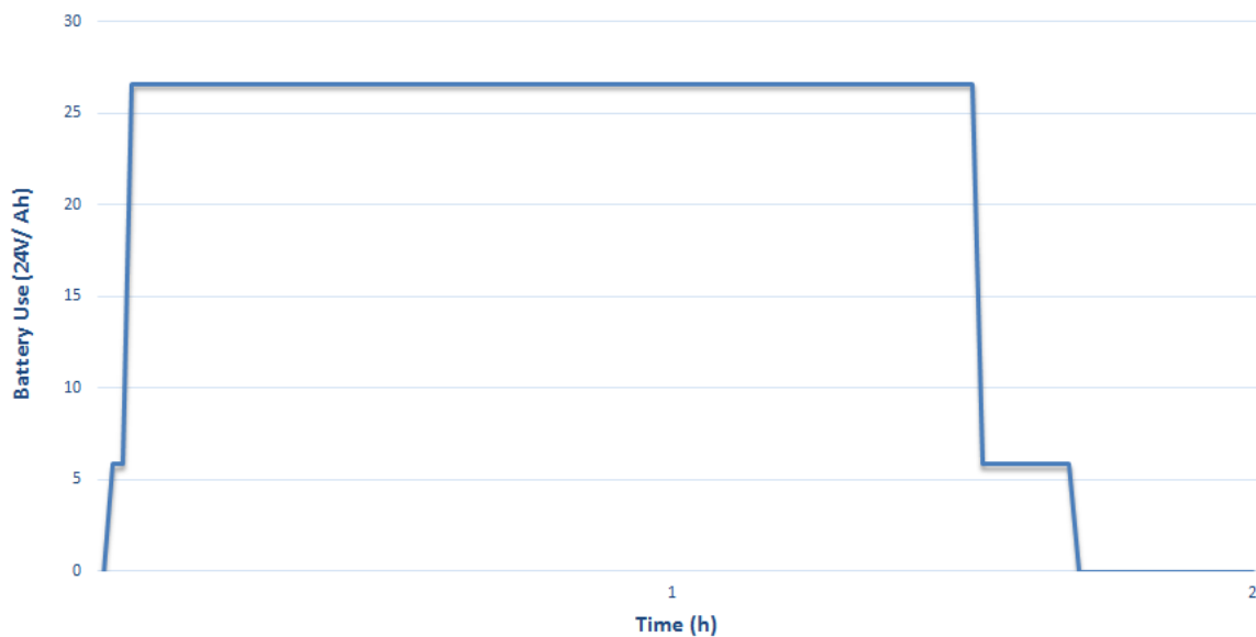
Figure 7.2 The ATS Firefighting Robot Operation in Concentrated Fire area
