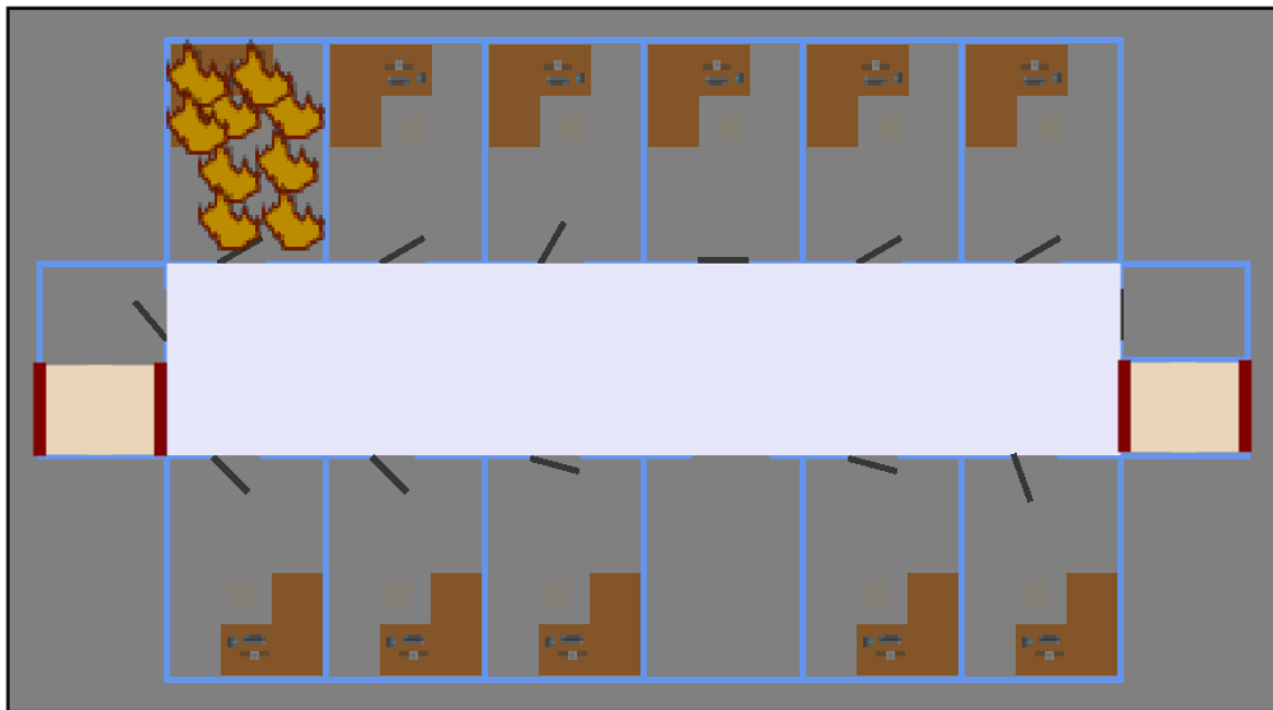
Figure 6.13 Fire spread for twenty minutes
