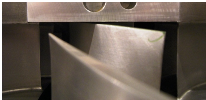
Figure 2.4: Missing 45 degree ramp upstream of Rotor 2, shown here for TC2. Flow is from left to right.
