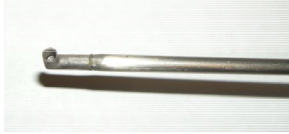
Figure 2.12: Fast-response total pressure probe.
