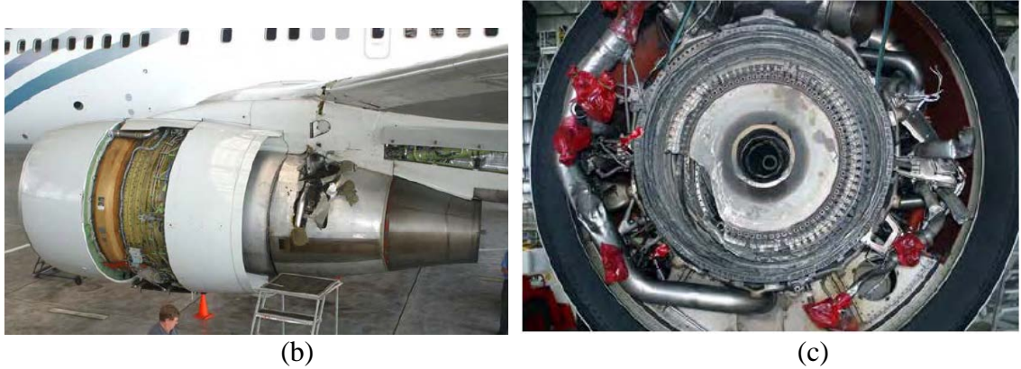
Figure 1.1. Uncontained high pressure turbine disc failure (a) in Boeing 767-223 on June 2, 2006 [8], (b, c) in Boeing 767-219ER on December 8, 2002 [9].
