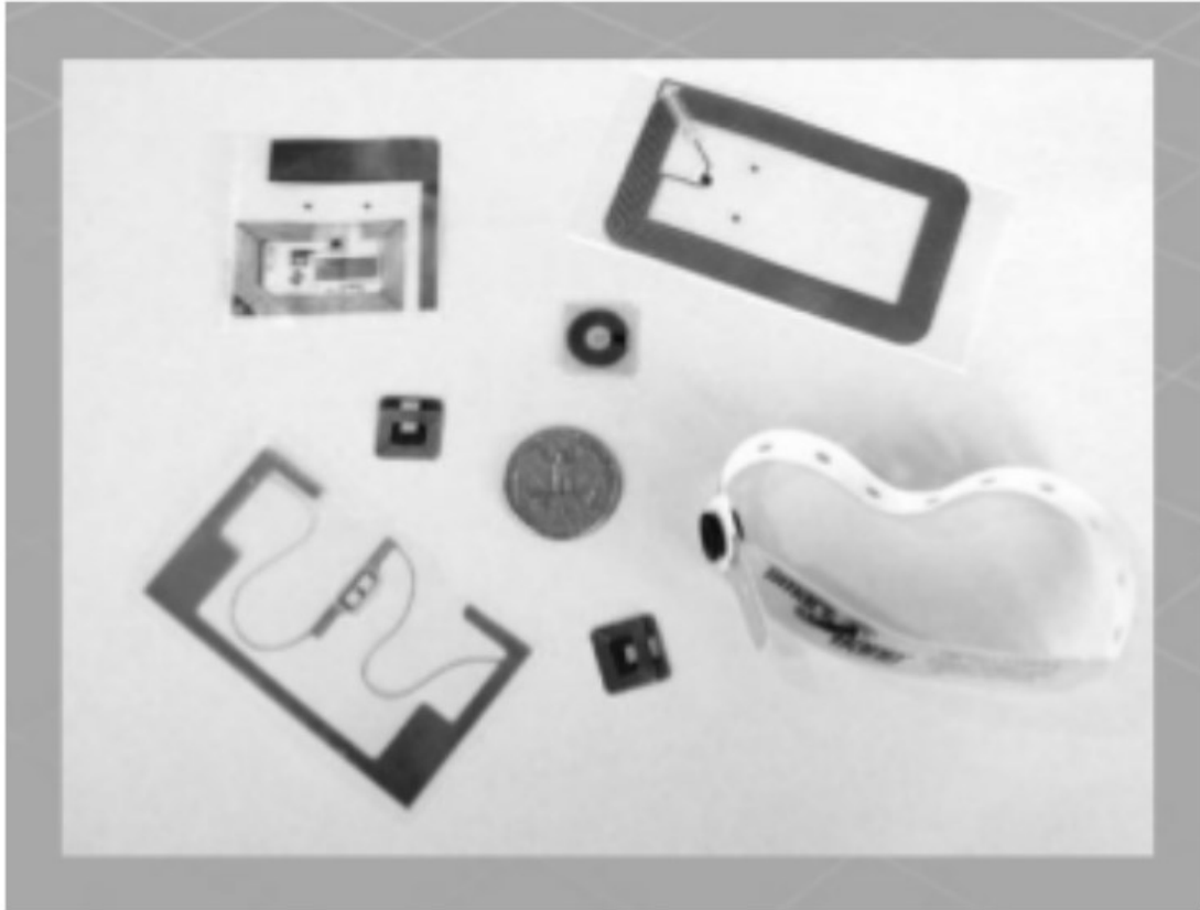
Figure 1 Popular RFID Tags in Various Shapes and Sizes (Want, 2004)
