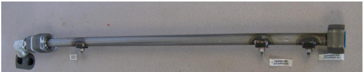
Figure 2.21: Calibrated steel pipe with embedded sensors.
