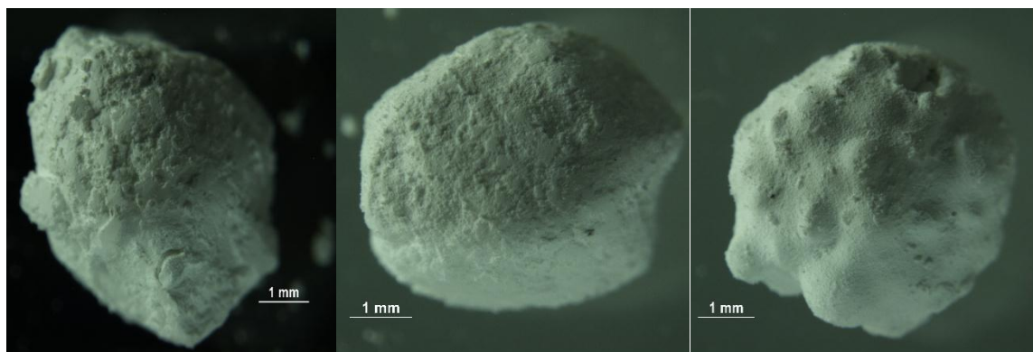
Figure 0.B.6: Optical Microscopy Powder A 10 minutes (A) 5.5 cP (B) 35 cP (C) 70 cP
