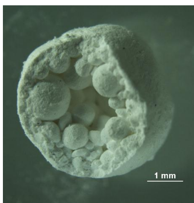
Figure 5.14: Powder A5, 15 minutes, broken shell showing hollow agglomerate structure
