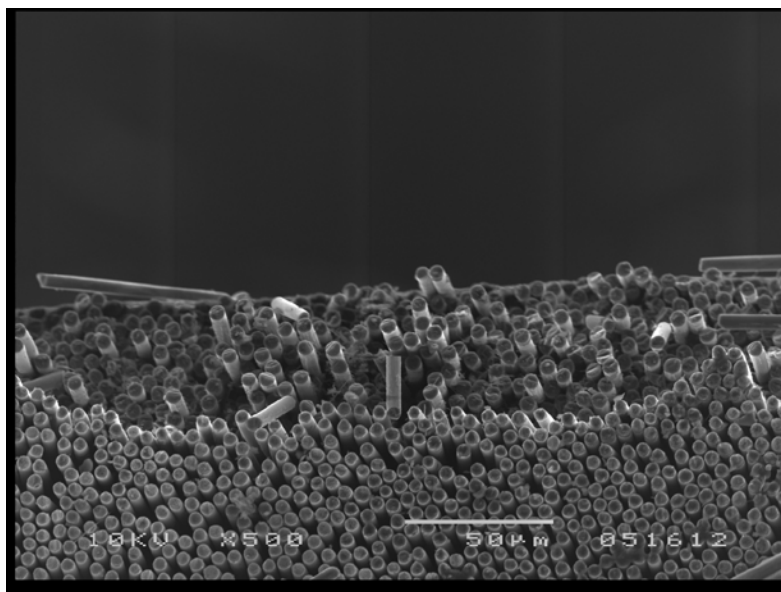
Figure 5.9. Broken fibers in the crater region (laser focus 1.0 mm away from target).
