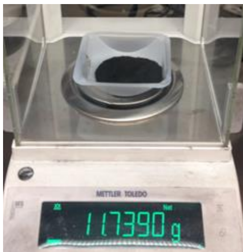
Figure 3.13 Purified, dry PbTe nanowire powder from one synthesis batch.
