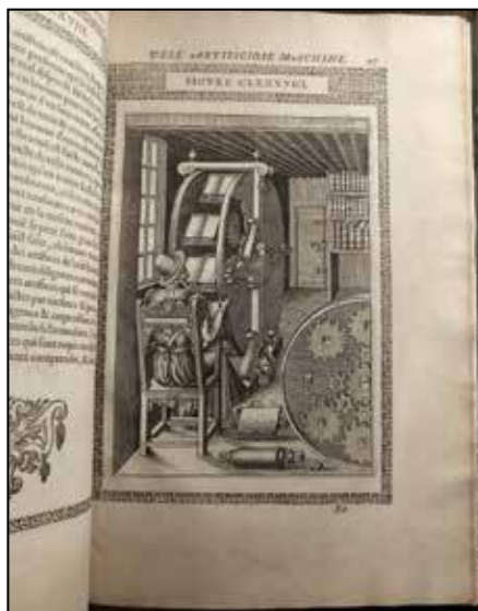
Photo Caption: Drawing from Le diverse et artificiose machine del capitano Agostino Ramelli ( The Varied and Ingenious Machines ), published in Paris, 1588. The machine shown here is a wheel-operated book-holding device for a scholar who suffers from gout. Rare Books and Special Collections Division, Library of Congress.
