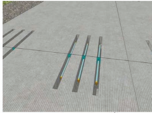
Load Transfer Retrofit b
