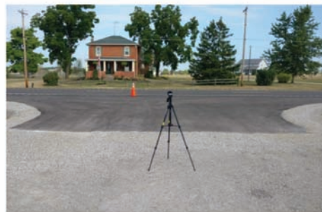
(c) Sound meter at distance of 50' off the edge line and at a height of 4' above ground level
