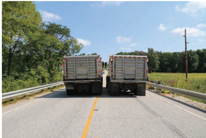
Figure 6.8 Two trucks static loading.
