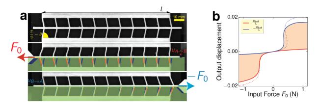
Fig. 1. Static Non-reciprocity in mechanical metamaterials. (a) Snapshots of the fishbone structure at rest (top), actuated from the left (middle) and from the right (bottom). The image difference has been overlaid on the bottom half of the pictures. (b) Output displacement vs. input force showing a strong non-reciprocal response (depicted by the shaded area). Adapted from [1].
