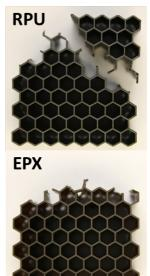
Figure 2: (Left) Example test data showing stress vs strain for two parts compressed in the X2 direction. The parts are printed from either EPX or RPU, with t/l = 0.20 and relative density of 0.23. (Right) Post compression samples in RPU and EPX.
