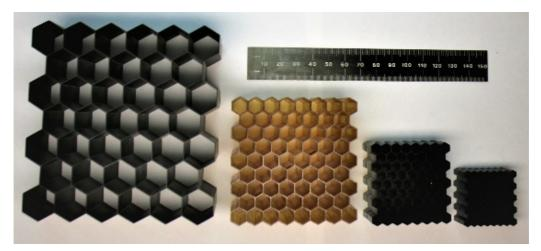
Figure 1: Hexagonal lattices printed using CLIP in four different materials (left to right) EPX, CE, RPU, and FPU at relative densities of 0.06, 0.12, 0.12, and 0.23 respectively. The ruler shows millimetres.
