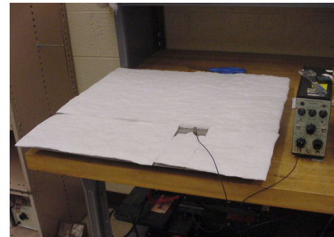
Test on Fibrous Dampers [4]
