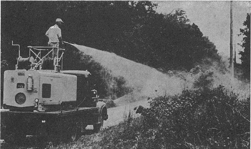
Fig. 3. Here is an efficient spraying operation on a county road. A mixture containing 2,4-D and 2,4,5-T is being sprayed from a fixed nozzle and a spray gun.
