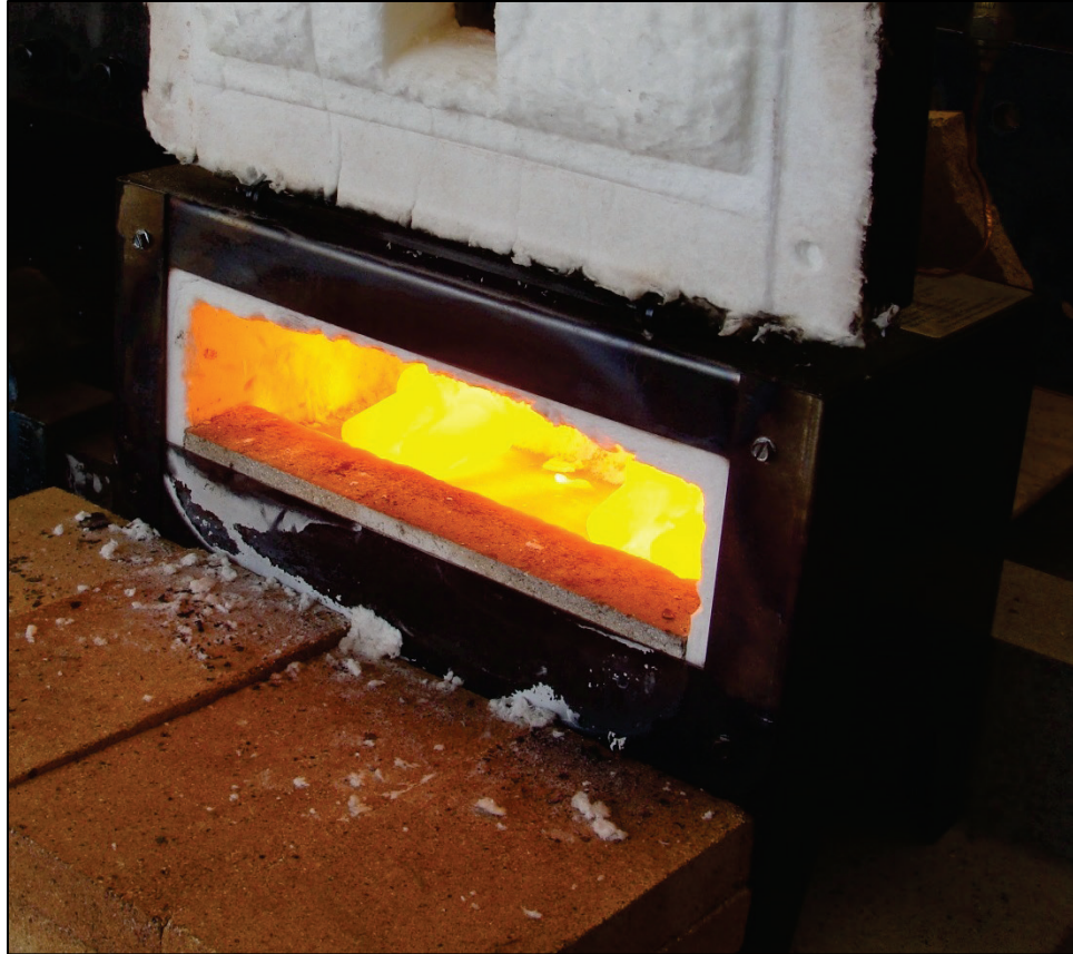
Figure 3-9 Propane fueled rivet forge
