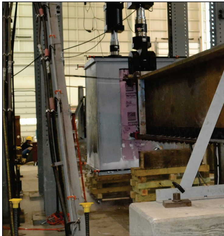
Figure 3-22 Temperature chamber installed on beam (end view)
