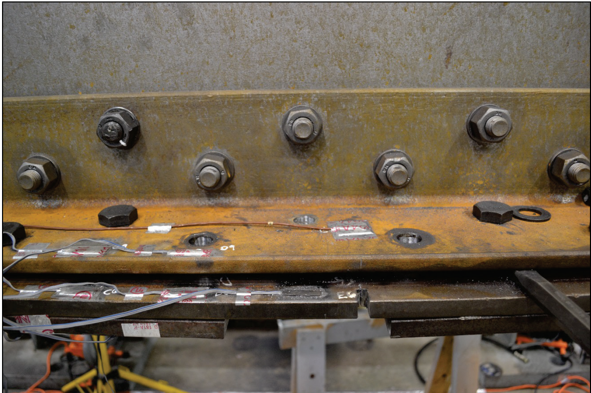
Figure 3-54 Specimen 36-2 notched upper cover plate
