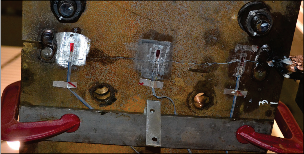
Figure 3-58 Specimen 46-4 fractured cover plate
