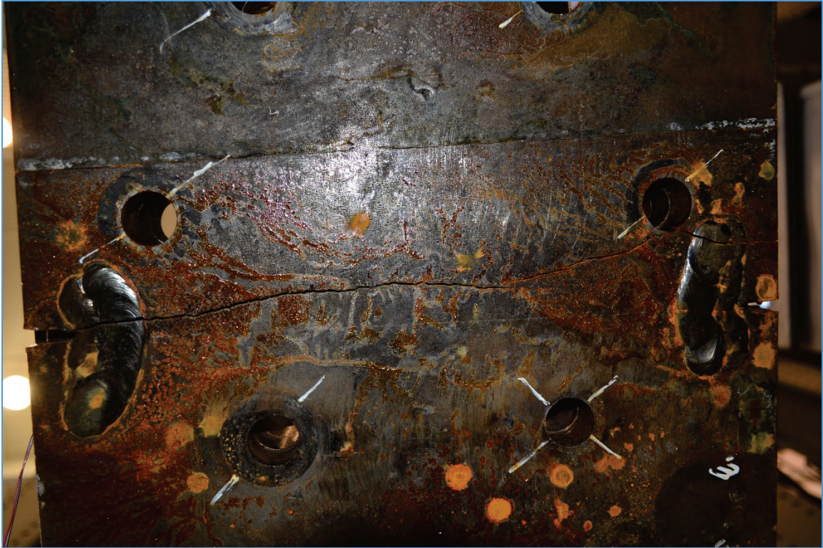
Figure 3-62 Specimen 36-4 fractured cover plate
