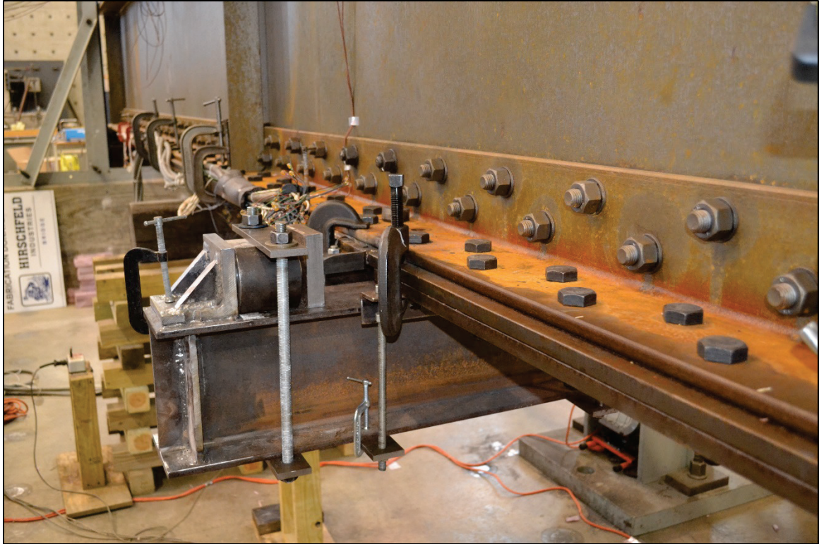
Figure 3-26 Driven wedge apparatus installed on Specimen 36-2
