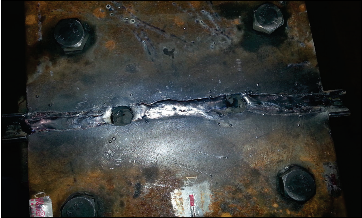
Figure 3-51 Specimen 36-2 welded lower cover plate
