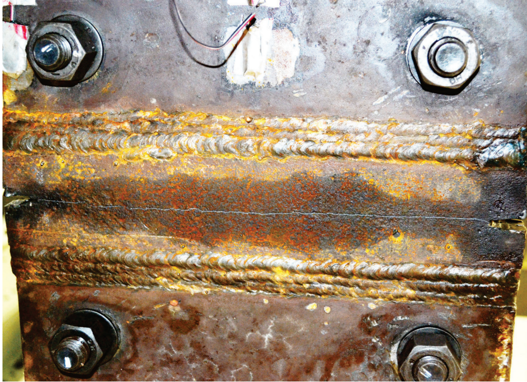
Figure 3-67 Specimen 30-1 fractured cover plate
