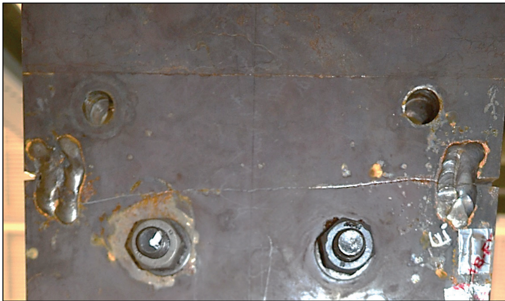
Figure 3-60 Specimen 36-3 fractured lower cover plate
