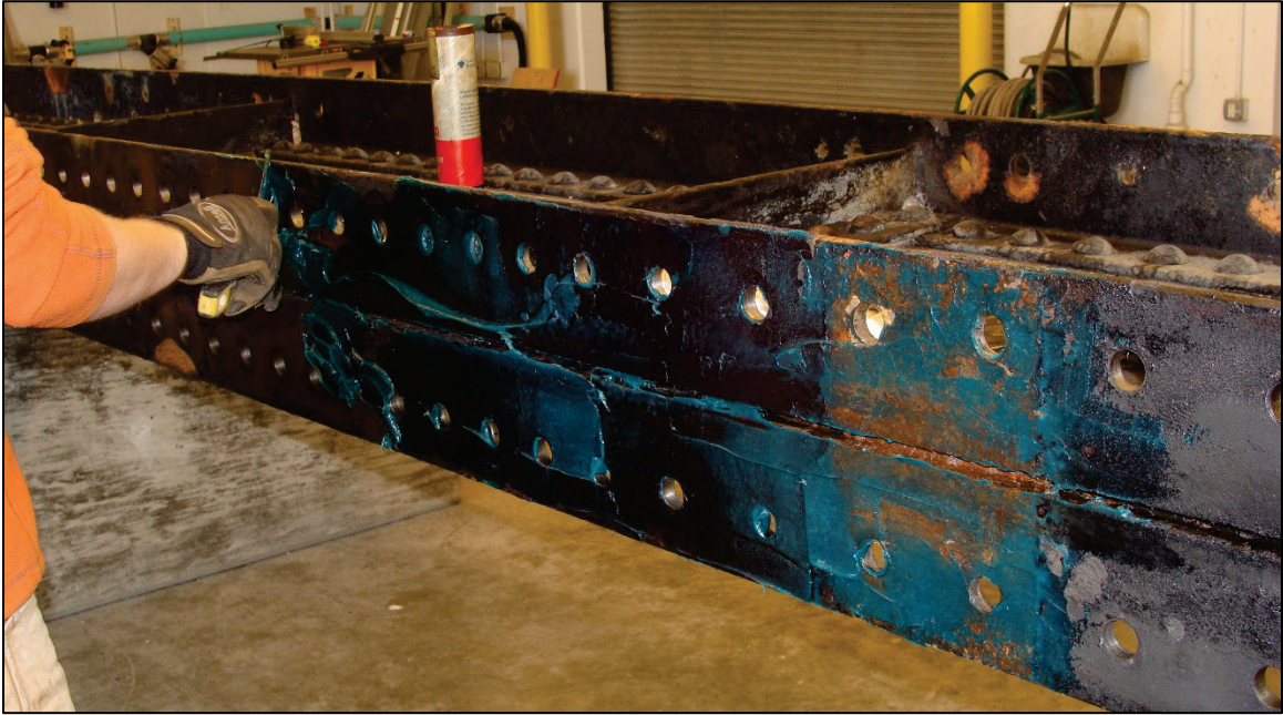
Figure 3-29 Specimen 23-1 application of grease between components
