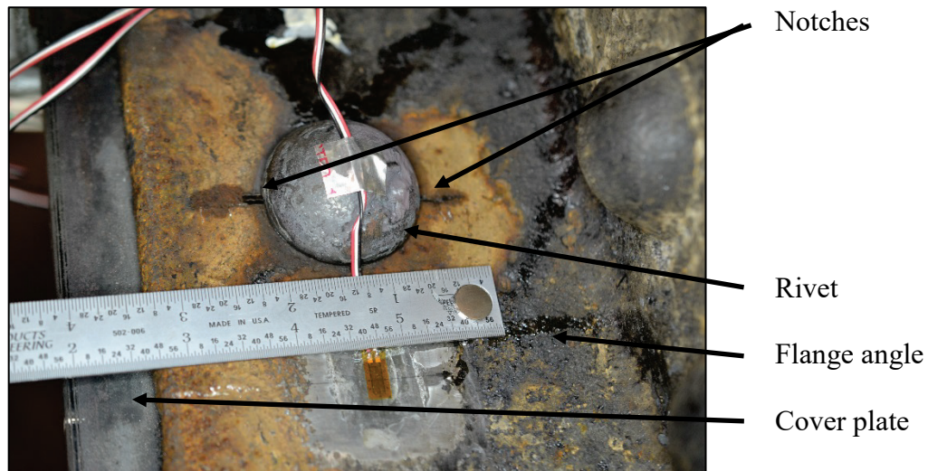
Figure 3-33 Specimen 23-2 hole notches
