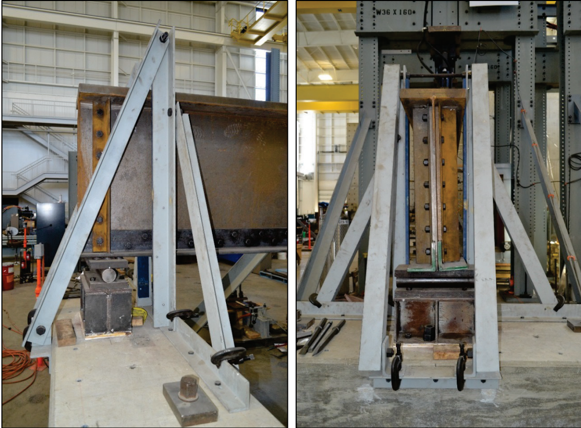
Figure 3-4 Lateral torsional bracing at specimen ends
