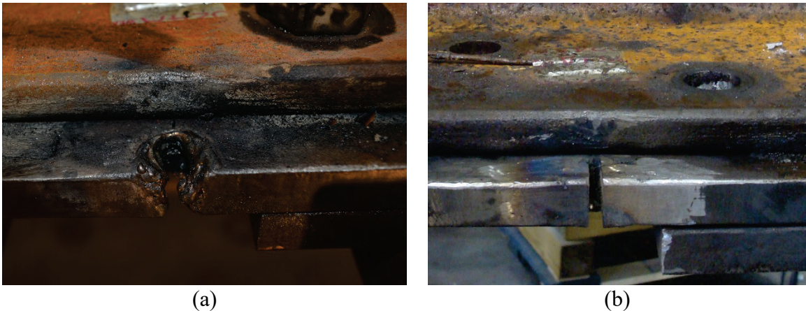
Figure 3-55 Specimen 36-2 upper cover plate notches (a) 2 nd attempt (b) 3 rd attempt
