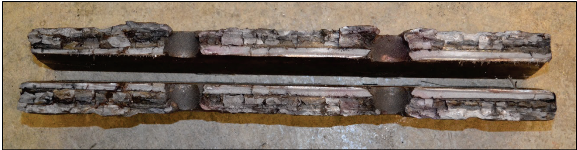
Figure 3-53 Specimen 36-2 lower cover plate failure surfaces
