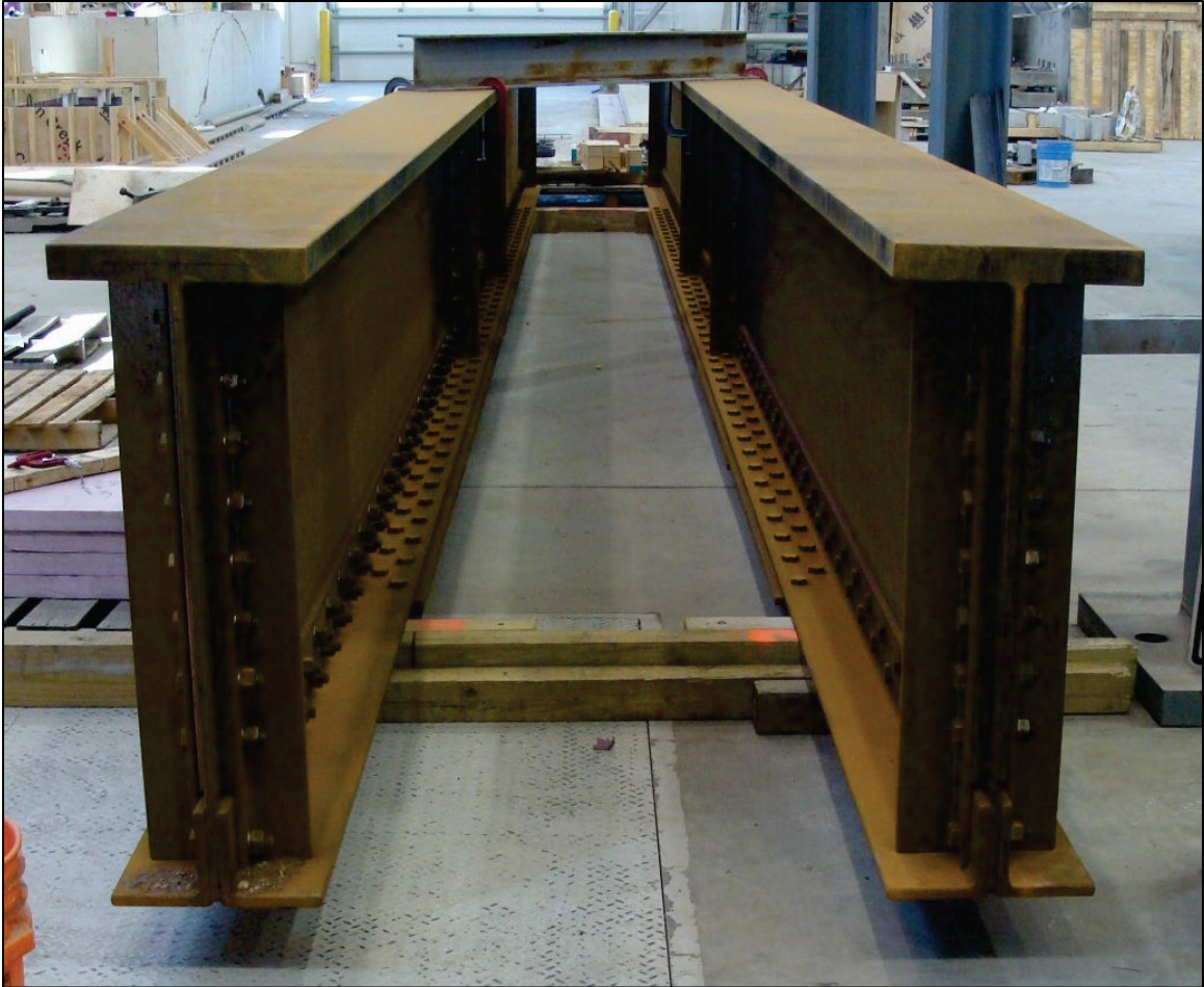
Figure 3-17 Fabricated Specimens (46" Web Height)
