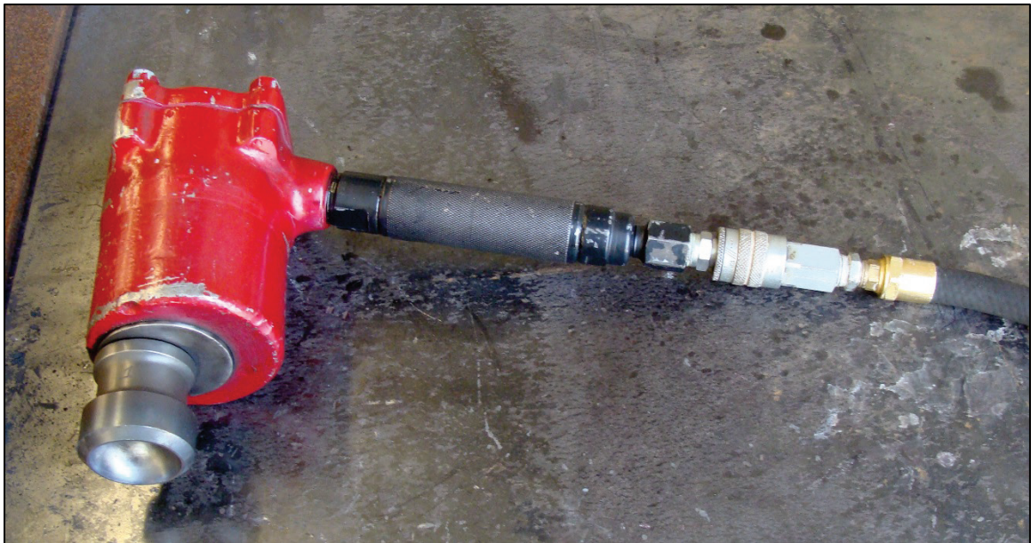
Figure 3-8 Chicago Pneumatic CP-AA-Offset holder-on
