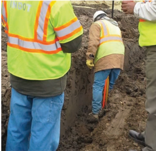
Figure C.5 Eight-inch rutting @ approximately 508+50.
