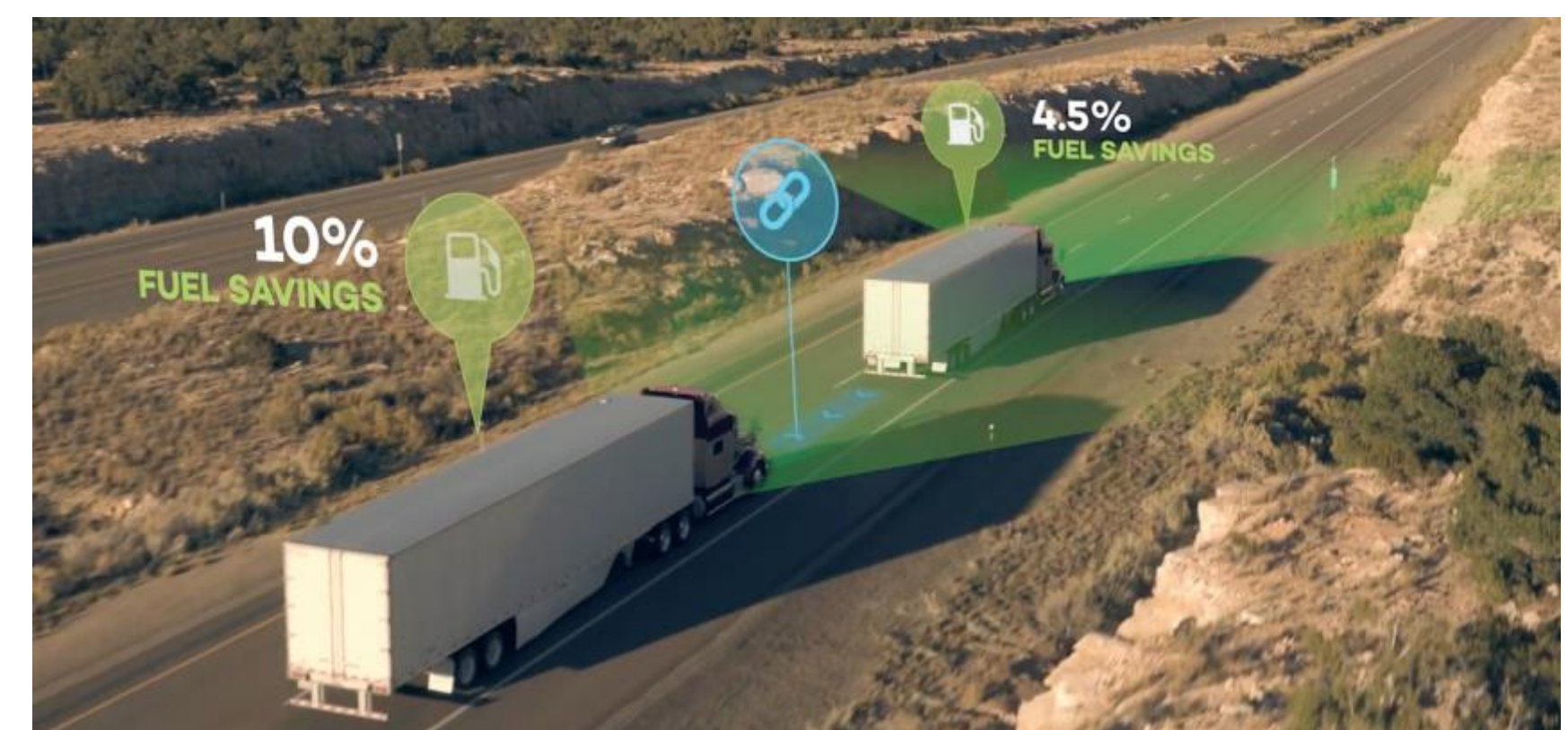
More efficient two-truck platooning using connectivity-enabled shifting coordination and lead truck predictive cruise
