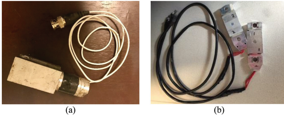
Figure 3.2 Transducers used in the PDCS: (a) accelerometer (b) strain transducer.
