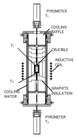
Figure 1. Schematic diagram of the inductively heated sublimation reactor.  $T_t$  and  $T_b$  refer to the top and bottom crucible temperatures, respectively.
