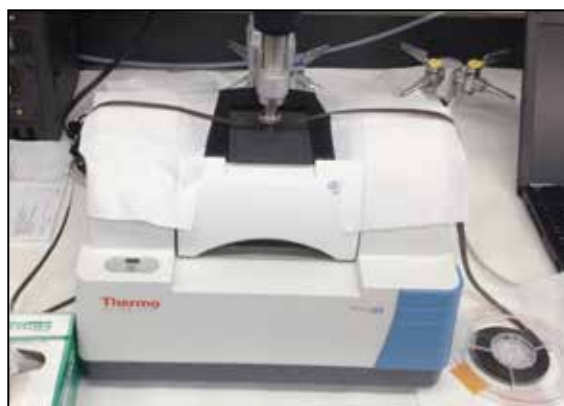
Figure 1. Infrared Analysis of a quarter-inch tape using a Portable Spectrometer.
