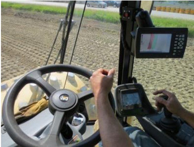
FIGURE 2 GPS MAPPING SYSTEMS CAN HELP OPERATORS VISUALIZE THE WORK IN REAL TIME
