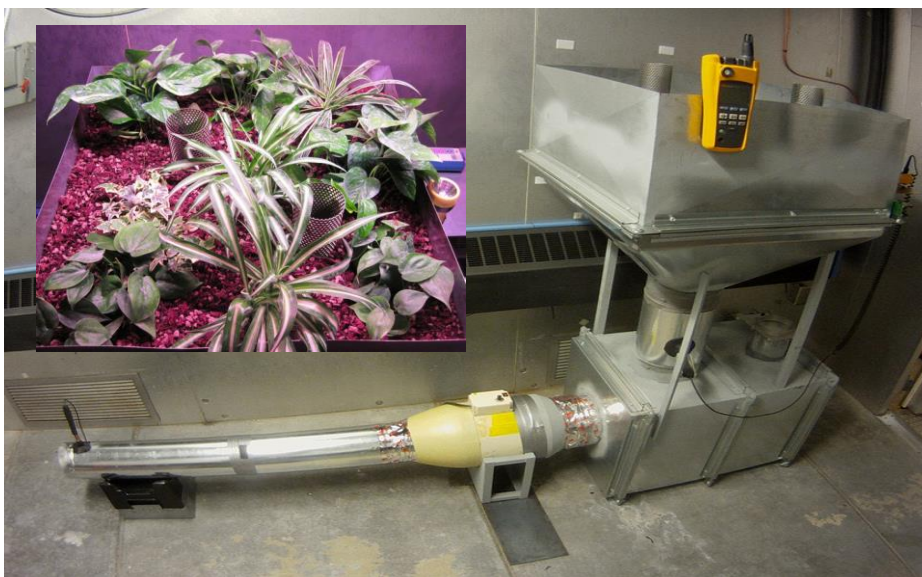
Figure 4. Biowall test apparatus in an environmental chamber.
