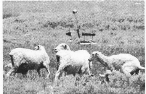
Figure 5. Sheep exhibited no response after triggering animal-activated acoustic frightening devices, which were designed to reduce coyote depredation, Wyoming, 2002.
