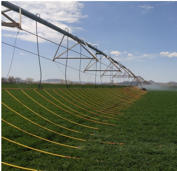
Figure 1. A Dragon-Line® mobile drip irrigation system on a center-pivot near Cedar City, UT. Note the misting on the spans in the background with mid-elevation i-wob sprinklers. Reduction in wind drift is one advantage of MDI.
