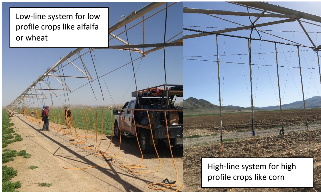
Figure 2. Installation of a Dragon-Line® low-line mobile drip irrigation system in a field near Cedar City (left) and a high-line system on a pivot near Elberta, Utah (right). Existing nozzles were cut off then the hoses were connected to manifolds and horizontal tubing supported by wire cabling. Drip tape was attached to the horizontal tubing at 30” inch spacing.
