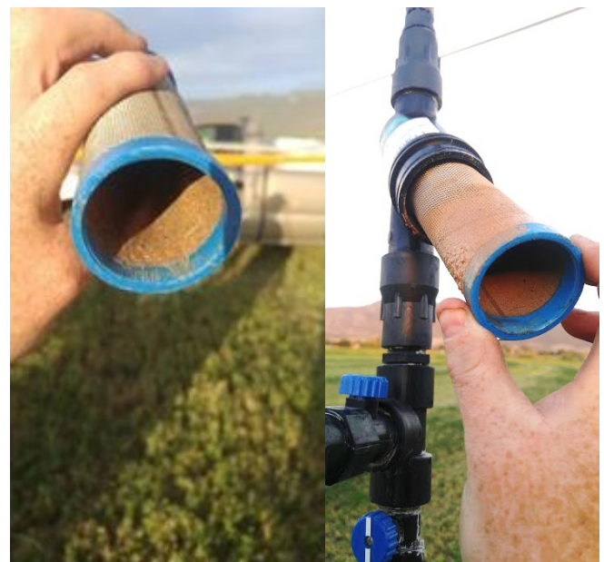
Figure 3. Small in-line 100 mesh spin clean filters above MDI systems in Utah showing sediment (left) and bacteria (right) contaminants. These filters were used for research applications and may not be feasible in production settings.
