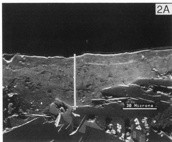
Figure 2. Rock varnish collected from a ca. 90 ka old lava flow (Turrin et al., 1985). Sample CIU-47. A) Backscattered electron SEM photomicrograph showing a consistently thick coat of varnish with a uniform surface. Note how relative thickness of varnish is related to the microtopography of original substrate surface.
