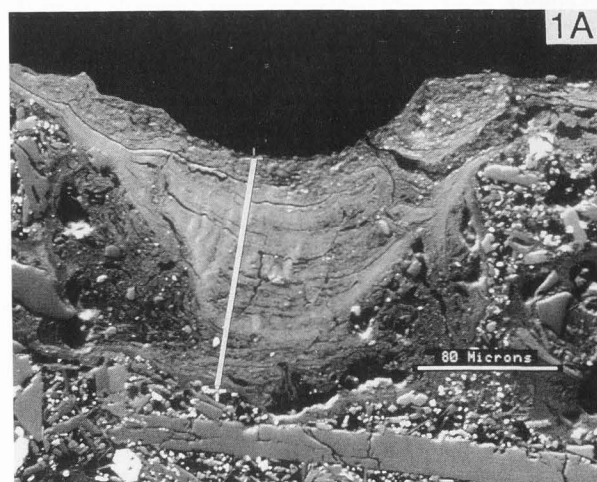
Figure 1. Rock varnish from a lava flow ca. 15-20 ka old (Wells et al., 1990). Sample CIA-16. A) Backscattered electron SEM photomicrograph showing brighter Mn-rich varnish and darker, detritus-rich varnish with visible foreign grains. The varnish is filling a depression on the substrate surface and is about 20x thicker in the depression than on the surrounding highs.
