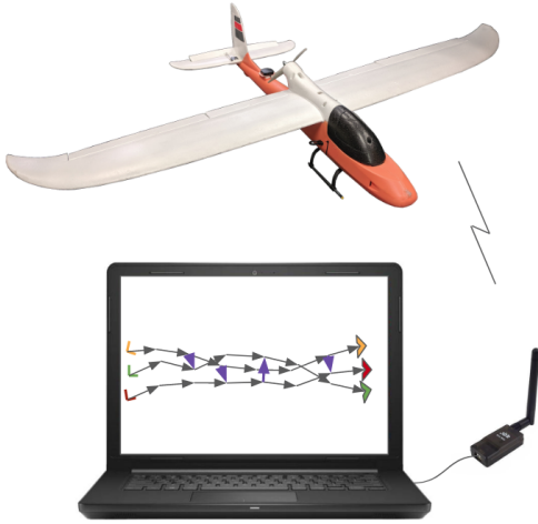
Fig. 5. Hardware tests of the complete system were performed on a STRIX StratoSurfer, RC-grade aircraft. The cooperative localization was tested with one complete agent and other agents utilizing recorded data from previous flights. This means that the communication was real and the test was completely realistic to the aircraft's perspective.
