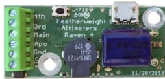
Figure 2. Picture of the RAVEN 4 Altimeter which will provide primary charge ignition and flight logging.
